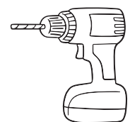
Drill and 1/8" Drill Bit
