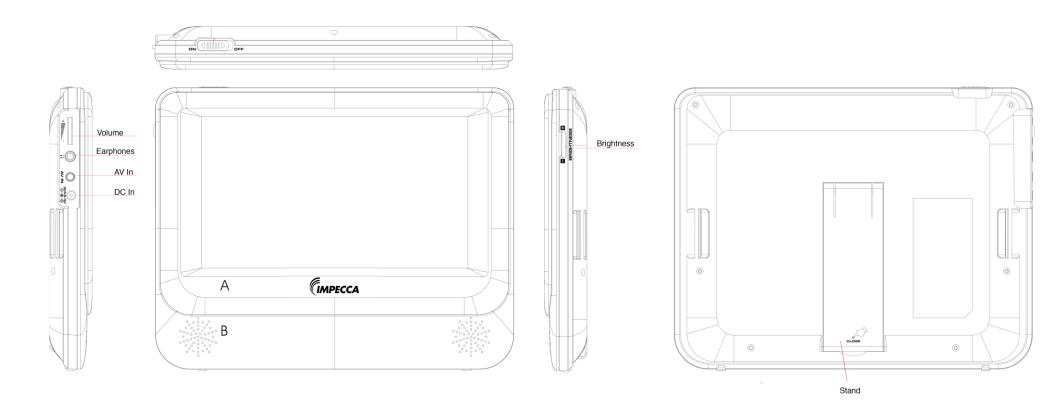
**DC In** - Plug in the DC cable (included) to power this screen **AV In** - Plug in the AV (Audio/ Video) cable (included) to connect this screen
