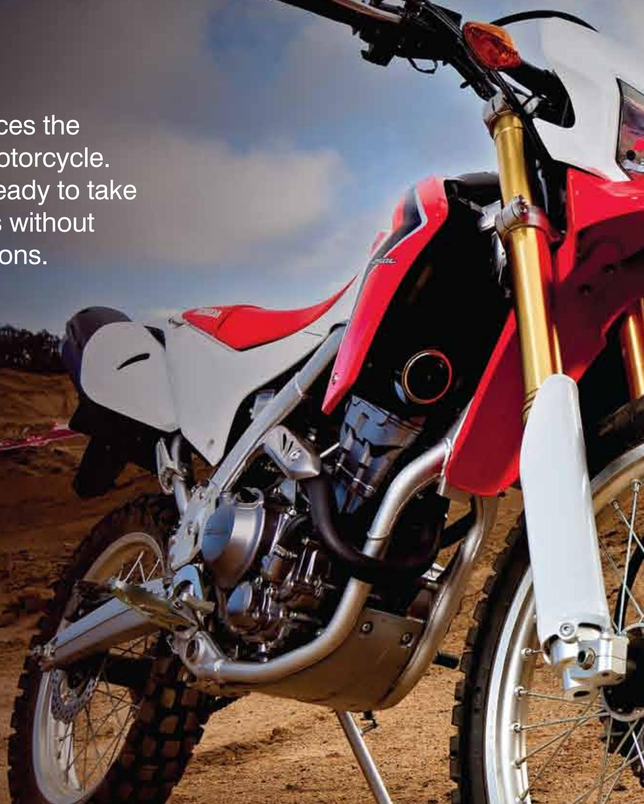
Compact and sophisticated liquid-cooled DOHC 249cc single-cylinder four-stroke powerplant produces smooth and consistent torque at low rpm to aid off-road work, yet the short-stroke engine also spins up excellent high-rpm performance for the street. The CRF250L pumps out a well-balanced and very capable level of power, along with excellent fuel economy. The CRF250L offers the full package, whether the day calls for low-cost transportation, a weekday commute or genuine dual-sport adventure.
