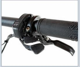
**XT Di2:** The Pinhoti Boost has an 11-speed electronic drivetrain that not only sounds cool in use, but also provides smooth shifting and a great range of gears.
