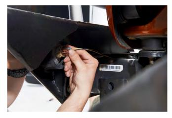
**STEP 7** // Route the fog light wiring above the frame rail and plug it back into the fog light housing.
