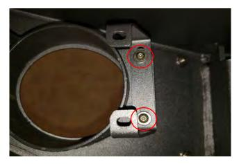
**STEP 5** // Install the supplied bracket to the barricade bumper and then install the fog lights onto the bracket and bumper by using the supplied M4 hardware.
