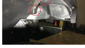
**Step 1**Using a panel removal tool, remove the (2) push clips holding the inner splash shield.
