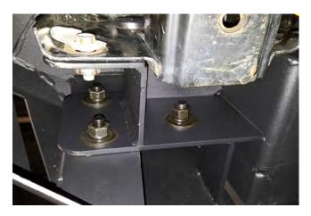
**STEP 7** // Slide bumper into place, and secure using the factory hardware.
