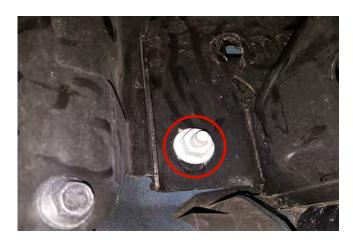
**STEP 3** // Unplug the factory fog light connectors and unclip the wiring harness from the bumper. Remove the lower (2) 21mm nuts. Then remove the front bumper from the vehicle. \*\*Note: Factory hardware will be reused.
