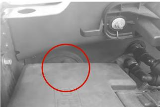
**STEP 12** // Optional LED light wiring, Route the on/off switch to the interior of the vehicle using a suitable body grommet. Mount the switch in the desired location. Zip tie any extra loose wiring away from heat and/or moving engine components.
