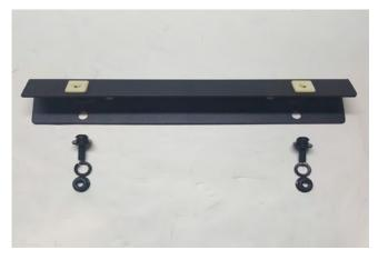
**STEP 4** // Attach the front license plate bracket to the new Barricade bumper if a front license plate is required using the (2) M6 screws, flat washers, and lock nuts.
