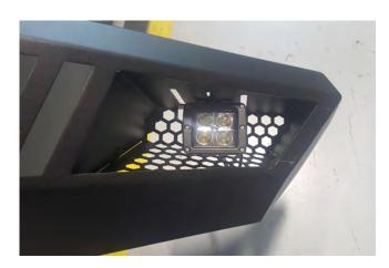
**STEP 9** // Optional LED light wiring, install the (2) LED lights into the middle slot of the bumper light housings using the supplied hardware.
