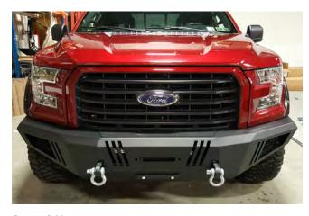
**STEP 8**// Install the (2) d-rings through the winch plate hooks.
