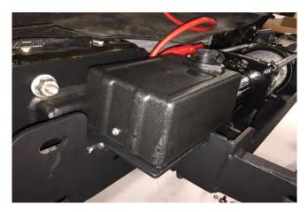
**STEP 6** // Attach the winch control box to the control plate mount using the (4) screws off the bottom of the control box.
