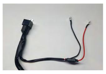
**STEP 11** // Optional LED light wiring, Install the Red 12+ volt wire to the positive battery terminal. Connect the black ground wire to the negative battery terminal. Mount the fuse in a safe location away from any damage that could occur. Tuck away any extra wiring.
