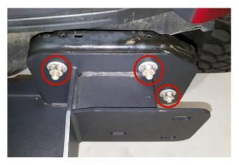
**STEP 5** // Install the winch plate to the frame of the vehicle using the factory hardware.
