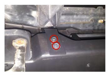
**STEP 7**// Install the (2) grille support brackets using (4) M8 x 25mm bolts, flat washers, and nuts.
