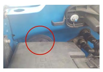
**STEP 14**// Optional LED Wiring: Route the on/off switch to the interior of the vehicle using a suitable body grommet. Mount the switch in the desired location. Safely secure any excess wiring out of the way.
