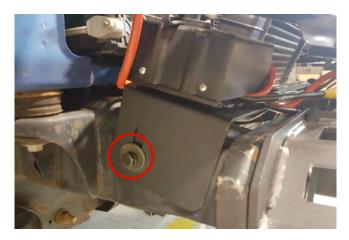
**STEP 6**// Install the control plate bracket to the frame using the M12x1.75x150mm bolt, (2) M12 flat washers, (1) M12 lock washer, and (1) M12 nut.
