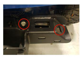
**STEP 4**// Attach the winch plate to the frame using (4) M12x1.75x45mm bolts, (8) M12 flat washers, (4) M12 lock washers, (4) M12 nuts, and (4) plastic holder washers.
