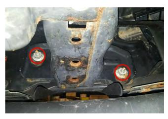
**STEP 3**// Next, disconnect the (2) Fog light harness if equipped. Loosen the (4) 21mm nuts holding the front bumper to the vehicle and then remove the bumper. \*\*Note: Factory hardware will not be reused.
