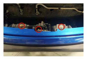
**STEP 10**// Reinstall the hood latch bracket using the factory hardware.
