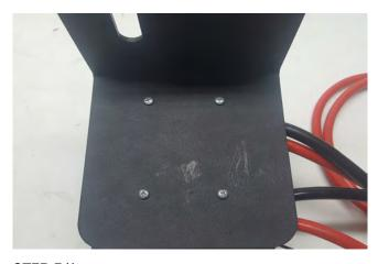
**STEP 5**// Attach the winch control box to the control plate mount using the (4) screws off the bottom of the control box.
