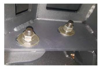
**STEP 8**// Slide bumper into place, and secure using (2) M12 double bolt plates, (4) M12 flat washers, (4) M12 lock washers, and (4) M12 nuts. \*\*Note: Be sure to center, and mount the bumper in the furthest up position.
