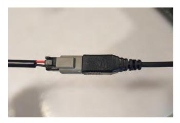
**STEP 12**// Optional LED Wiring: Connect the supplied wiring harness to the LED lights. Be sure to zip tie the excess wiring away from hot/moving engine bay components.
