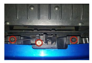
**STEP 2**// Remove the (2) 8mm screws, and (1) 10mm bolt that hold the hood latch plate to the factory bumper lip. \*\*Note: Factory hardware will be reused.
