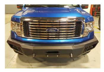
**STEP 9**// If required attach the license plate bracket using the (2) M6 screws, lock washers, and nuts.
