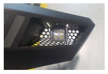
**STEP 11**// Optional LED Lighting: Install the (2) LED lights into the middle slot of the bumper light housings using the supplied hardware.
