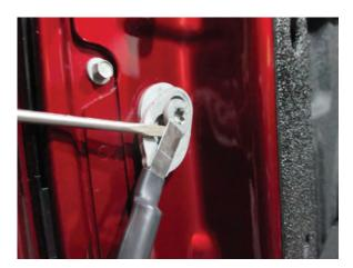
Step 1\\ Remove the lift gate strap and loosen the T50 lift gate bolt.
