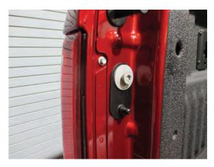
Step 2\\ Install the upper bracket behind the upper lift gate bolt. Reinstall lift gate strap.
