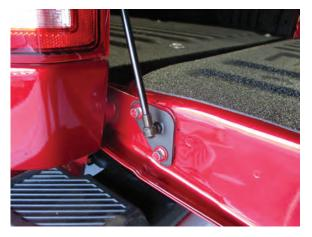
Step 4\\ Install the lower ball mount plate, reuse the factory bolts.
