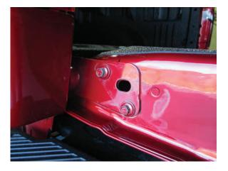
Step 3\\ Remove the (2) 10mm bolts on the lower tailgate bracket.
