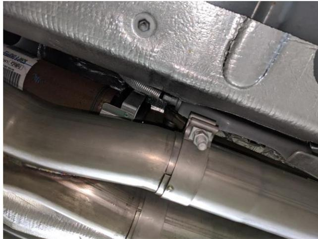
7. Install driver and passenger side tailpipes using (2) 3" clamps, one for each side.
