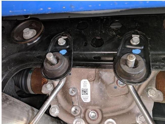
4. Remove the exhaust from the hangers and remove from vehicle. Hangers by the rear bumper, held in by (2) 13mm bolts, can be removed to make removal easier if needed. Recommended to have 2 people for this step.
