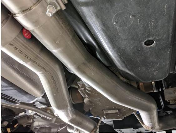
8. Install driver and passenger side mufflers into the rear hangers and onto the tailpipes using (2) 3" clamps, one for each side.
