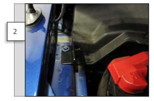
Install bracket marked P-L using factory fender bolt as shown.
