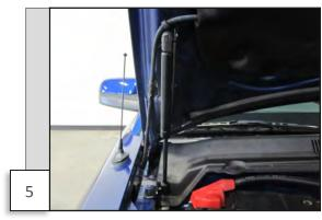
Pop the ends of the strut over the ball mounts on the brackets. Repeat steps 1-5 for drivers side. *(do not slam hood shut yet)* Check bumper/fender alignment by slowly lowering the hood. If okay, remove factory prop rod and enjoy.
