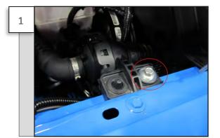
Remove the bolt holding the canister bracket to the inner fender. Also remove the factory u-nut from the fender for reuse.
