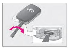
**3** Remove the depleted battery.
