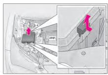
► Engine compartment: type B fuse box
