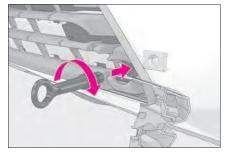
**4** Tighten down the towing eyelet securely using a wheel nut wrench.
