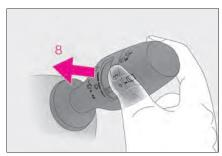
8 Washer/wiper dual operation The wipers will automatically operate a couple of times after the washer squirts. Vehicles with headlight cleaners: When the headlights are on and the lever is pulled and held, the headlight cleaners will operate once. After this, the headlight cleaners will operate every 5th time the lever is pulled.
