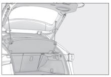
Pull the lever upwards and open the deck board.
