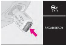
Accelerate or decelerate, with accelerator pedal operation, to the desired vehicle speed (at or above approximately 30 mph (50 km/h)) and push the lever down to set the speed.
