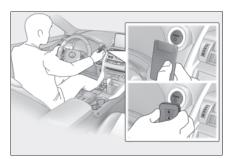
Firmly depress the brake pedal and check that message shown on the multi-information display.
