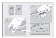
Grip the driver's door handle to unlock the door. Grip any passenger door handle to unlock all the doors.\*
