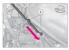
5 Holding a rag under the end, pull the dipstick out and check the oil level.
