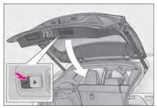
Close the back door and lock all doors (close & lock function)
