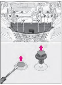
■ Installing the clips
