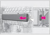
5 Remove the air conditioning filter and replace it with a new one.
