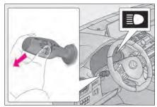
Press the Automatic High Beam switch.
