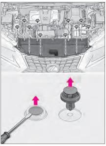
■ Installing the clips
