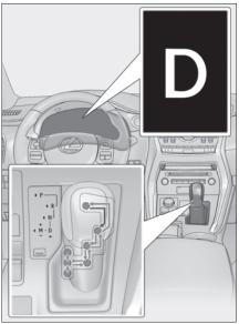
While the engine switch is in IGNI-TION ON mode, move the shift lever with the brake pedal depressed. When shifting the shift lever between P and D, make sure that the vehicle is completely stopped.
