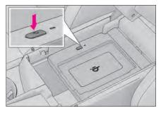
3 Place the charging side of the portable device down.
