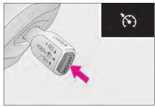
2 Accelerate or decelerate, with accelerator pedal operation, to the desired vehicle speed (at or above approximately 25 mph [40 km/h]) and push the lever down to set the speed.
