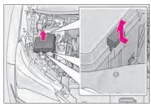
► Engine compartment: type B fuse box
