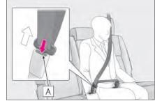
Insert the mechanical key (→P.86) or plate B into the notch of buckle and remove the belt.
