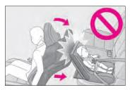
Do not allow the child to lean his/her head or any part of his/her body against the door or the area of the seat, rear pillars or roof side rails from which the SRS curtain shield airbag deploys even if the child is seated in the child restraint system. It is dangerous if the SRS curtain shield airbag inflates, and the impact could cause death or serious injury to the child.
