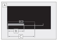
A Eco Driving Indicator Zone Display Suggests the Zone of Eco driving with current Eco driving ratio based on acceleration.
