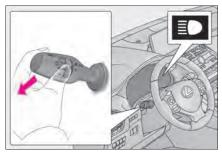
2 Press the Automatic High Beam switch.
