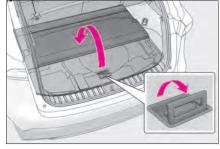
3 Lift the deck board and remove the hook on the backside of the deck board.
