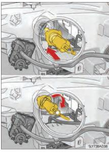
**8** Confirm the installation of the bulb base.
