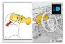
2 Press the Automatic High Beam switch.
