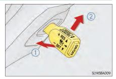
However, resuming is available when the vehicle speed is more than approximately 25 mph (40 km/h).
