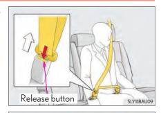
Insert the mechanical key (→P.122) or plate B into the notch of buckle A and remove the belt.
