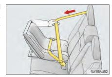
SWhile pushing the child restraint system down into the rear seat, allow the shoulder belt to retract until the child restraint system is securely in place.
