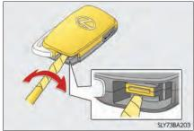
Remove the depleted battery.
