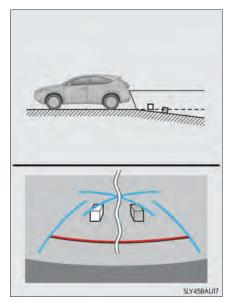
• When any part of the vehicle sags When any part of the vehicle sags due to the number of passengers or the distribution of the load, there is a margin of error between the guide lines on the screen and the actual distance/course on the road.
