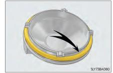
6 Replace the light bulb, and set the connector
