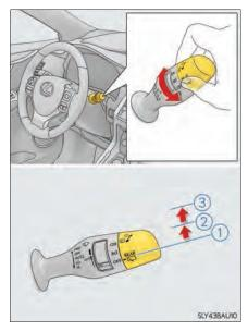
Washer/wiper dual operation The wipers will automatically operate a couple of times after the washer squirts.
