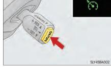
2 Accelerate or decelerate, with accelerator pedal operation, to the desired vehicle speed (above approximately 25 mph [40 km/h]) and push the lever down to set the speed.
