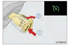
When in constant speed control mode, to return to vehicle-to-vehicle distance control mode, push the lever forward again and hold for approximately 1 second.
