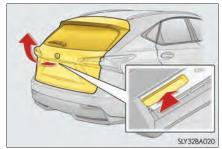
While carrying the electronic key on your person, press the back door opener switch.
