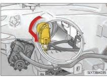
4 Unplug the connector while pulling the lock release.
