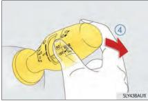
■ The rear window wiper and washer can be operated when The power switch is in ON mode.
