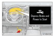
4 Press the power switch shortly and firmly.
