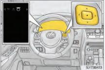
Press or v of the meter control switch, select the "TPMS" screen and then press and hold the □.
