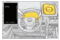
7 A message and an indicator are displayed by the multi-information display, and initialization is completed.
