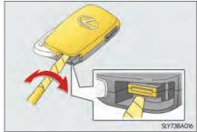
Remove the depleted battery.
