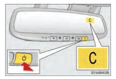
3 Drive the vehicle at 5 mph (8 km/h) or less in a circle until a direction is displayed.
