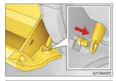
Push in the glove box on the vehicle's outer side to disconnect the claws. Then pull out the glove box and disconnect the lower claws.
