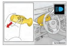
**2** Press the Automatic High Beam switch.
