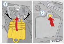
**9** Install the engine compartment cover.  $(\rightarrow P. 503)$
