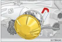
When removing the washer fluid supply opening:
