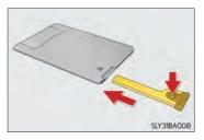
If the battery cover is not installed and the battery falls out or if the battery was removed because the key got wet, reinstall the battery with the positive terminal facing the Lexus emblem.
