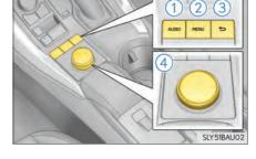
Move the controller to display the left or right side of the screen.
