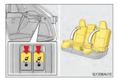
2 Check that the plate for the seat belt is on the front side of the seat.
