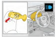
**2** Press the Automatic High Beam switch.
