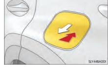
**2** Turn the fuel tank cap slowly to remove it and put it into the holder on the fuel filler door.
