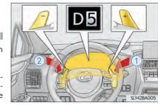
To return to normal D position driving, the "+" paddle shift switch must be held down for a period of time.
