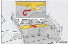
**5** Stow the luggage cover in the deck under tray while lifting the deck board.
