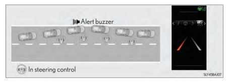
If the system judges that the vehicle has deviated from the current traffic lane, it is displayed in the multi-information display and steering force is supplied to the steering wheel by the steering control, providing required assistance in steering wheel operation to avoid further deviation from the marker lines.
