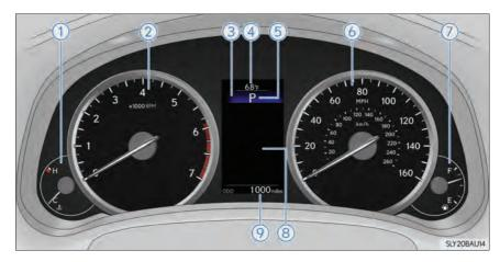
1) Engine coolant temperature gauge
