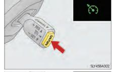
Accelerate or decelerate, with accelerator pedal operation, to the desired vehicle speed (above approximately 25 mph [40 km/h]) and push the lever down to set the speed.
