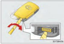
Remove the depleted battery.
