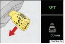
While the vehicle is in vehicle-to-vehicle distance control mode, if the lever is released when vehicle speed is less than 30 mph (50 km/h) and a vehicle ahead can be detected, the vehicle will start following the vehicle ahead at a set speed of 30 mph (50 km/h).
