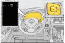
Press or of the meter control switch, select the "TPMS" screen and then press and hold the ...
