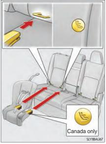
**5** After installing the child restraint system, rock it back and forth to ensure that it is installed securely.
