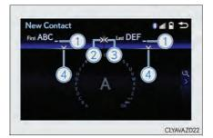
4 When this indicator is shown, you can change to input mode by moving the controller backward.
