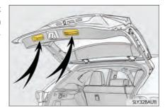
Vehicles with a power back door Lower the back door using the back door handle, then a buzzer sounds and the back door automatically closes.
