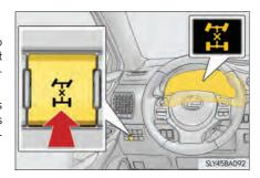
■ All-wheel drive lock mode can be operated when The engine switch is in IGNITION ON mode.
