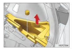
Remove the 12-volt battery maintenance cover.
