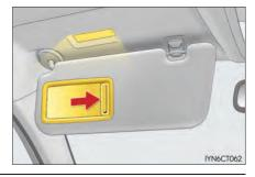
If the vanity light remain on when the power switch is turned off, the light will go off automatically after  $20\,\mathrm{minutes}$ .
