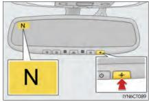
To turn the compass on or off, press the button.
