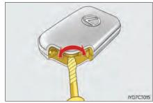
Remove the depleted battery.
