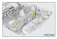
The portion of the front pillars, rear pillars or roof side rail garnishes (padding) containing the curtain shield airbags inside is scratched, cracked, or otherwise damaged.
