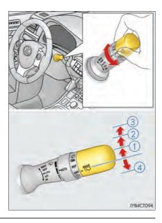
■ The rear window wiper and washer can be operated when The power switch is in ON mode.
