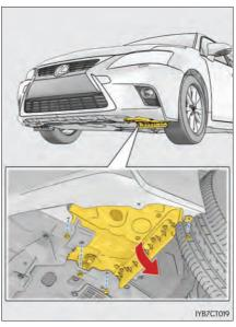
**2** Unplug the connector while pressing the lock release.
