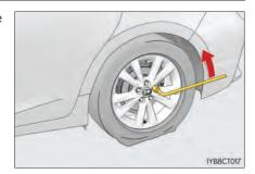
3 Turn the tire jack portion (A) by hand until the notch of the jack is in contact with the jack point.
