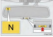
To turn the compass on or off, press the "AUTO" button for more than 3 seconds.
