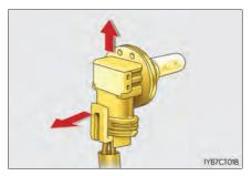
4 Replace the light bulb, and install the bulb base.
