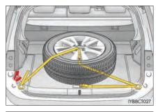
Pass the belt through the buckle and secure the tire firmly. Check that the belt is securely held by the buckle.
