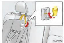
**3** Outboard only: Adjust the head restraint to the downmost position.
