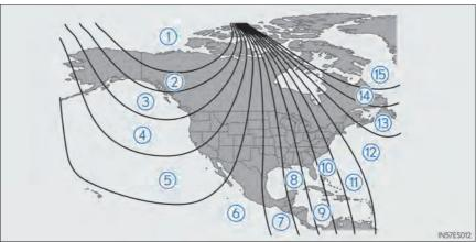
The direction display deviates from the true direction determined by the earth's magnetic field. The amount of deviation varies depending on the geographic position of the vehicle.
