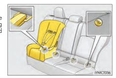
Seat belts equipped with a child restraint locking mechanism (ALR/ ELR belts except driver's seat belt)  $(\rightarrow P.34)$
