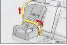
If the child restraint has a top tether strap, the top tether strap should be latched onto the top tether strap anchor.  $(\rightarrow P. 68)$
