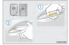
2 Touch the lock sensor (the indentation on the upper part of the front door handle) to lock the doors.
