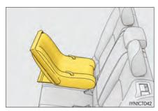
2 Run the seat belt through the child restraint system and insert the plate into the buckle. Make sure that the belt is not twisted.
