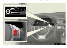
Press the "DISP" switch on the steering wheel several times to select the energy monitor display.
