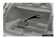
A part of the center auxiliary box can be used as an Owner's Manual holder.
