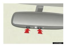
Press and hold the 2 outside buttons shown in the illustration for 10 seconds until the indicator light flashes.
