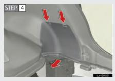
Remove the 12-volt battery maintenance cover.
