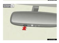
Press and hold the programmed HomeLink® button (located inside the vehicle) for 2 seconds and release it. Repeat this sequence (press/hold/release) up to 3 times to complete programming.
