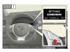
Press the "DISP" switch to display the "SETTINGS" screen while the vehicle is stopped, and then press and hold the "DISP" switch to display the customize mode screen.
