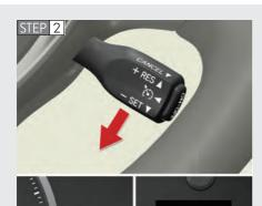
Accelerate or decelerate the vehicle to the desired speed, and push the lever down to set the speed.
