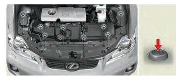
■ Installing the clips
