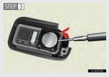
Remove the depleted battery.
