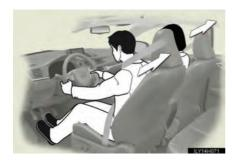
The pretensioner helps the seat belt to quickly restrain the occupant by retracting the seat belt when the vehicle is subjected to certain types of severe frontal or side collision and severe side collision.
