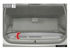
Fold the rear edge of the cover over, replace the side deck boards and close the center auxiliary box.
