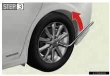
Slightly loosen the wheel nuts (one turn).
