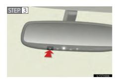
Test the HomeLink<sup>®</sup> operation by pressing the newly programmed button and observing the indicator light:
