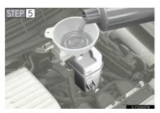
Add power control unit coolant if necessary.
