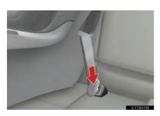
Press the buckle release button and fully retract the seat belt.
