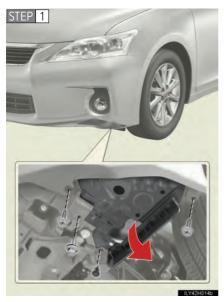
Remove 2 screws, a bolt and clip, and pull down the engine under cover.
