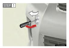
Remove the eyelet cover using a flathead screwdriver.
