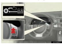
Push the "DISP" button on the steering wheel several times to select the energy monitor display.
