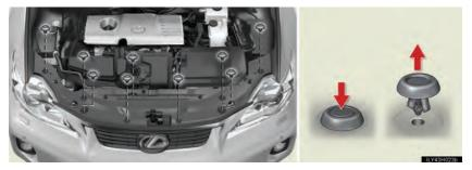
■ Installing the clips
