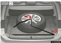
Place the flat tire on the deck board, and pass the belt through the lower-right cargo hook and then through the hole in the center of the tire.
