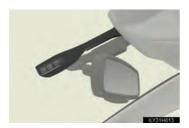
A sensor, which detects humidity inside the vehicle and the temperature of the windshield, is provided to detect fog on the front windscreen. Due to the sensor, when automatic mode is set the air conditioning may make the following controls:
