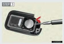
Remove the depleted battery.
