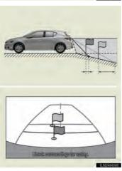
When the grade behind the vehicle slopes down sharply, objects appear to be closer than they actually are.
