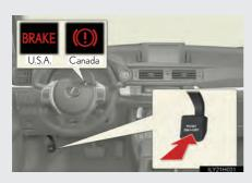
To set the parking brake, fully depress the parking brake pedal with your left foot while depressing the brake pedal with your right foot.
