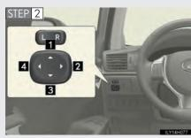
To adjust the mirror, press the switch.
