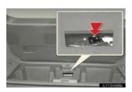
Lift the center deck board and then push down the lever in the hole.
