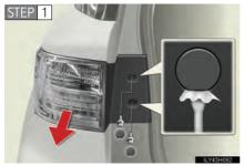
Open the back door and remove the covers and bolts, and remove the lamp assembly by pulling it directly backward from the rear of the vehicle.
