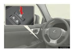
Press the switch down to lock the passenger window.
