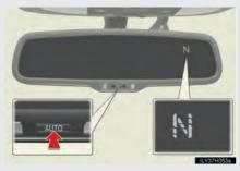
To turn the compass on or off, press "AUTO" button for more than 3 seconds.
