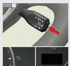
Press the "ON-OFF" button to activate the cruise control.
