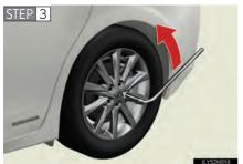
Slightly loosen the wheel nuts (one turn).
