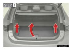
Remove the side deck boards and open the center auxiliary box.
