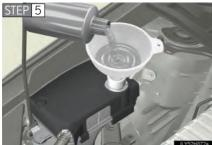
Add engine coolant if necessary.
