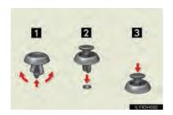
After lifting up the air cleaner duct or removing the power control unit cover, return the duct or the cover to their original positions with the clips.
