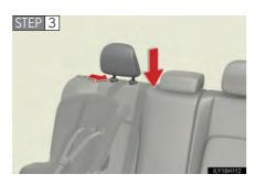
Outside only: Adjust the head restraint to the downmost position.
