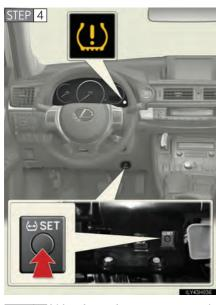
Press and hold the tire pressure warning reset button until the tire pressure warning light blinks slowly 3 times.
