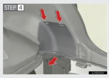
Remove the 12-volt battery maintenance cover.
