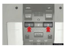
Press and hold the 2 outside buttons for 10 seconds until the indicator light flashes.
