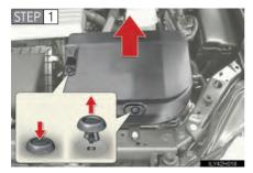
Remove the power control unit cover.
