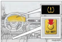
When position of each tire is determined, the inflation pressure of each tire will be displayed on the multi-information display.
