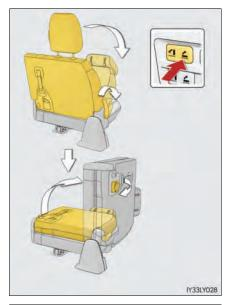
Remove the seat hook covers from the underside of the seat cushion, and install them on the seat hooks.
