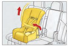
6 If the child restraint system has a top tether strap, the top tether strap should be latched onto the top tether strap anchor.  $(\rightarrow P. 69)$
