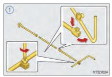
② Assemble the jack handle extension bar and the jack handle bar and tighten the bolts.
