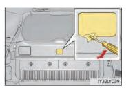
2 Push the lever for the back door motor, open the back door.
