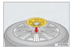
1 Install the holding bracket, inserting the claw into the wheel lug nut hole. Turn the jack handle extension clockwise to take up slack in the chain.
