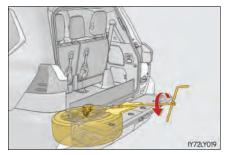
**5** Pull out the spare tire and remove the holding bracket and spare wheel cover.
