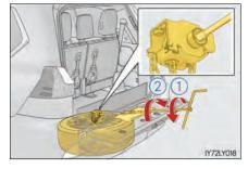
4 Lower the spare tire completely to the ground.
