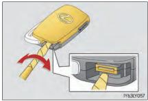
3 Remove the depleted battery.
