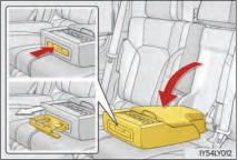
To open, pull down the armrest, press the button and release the rear cup holder on the armrest.
