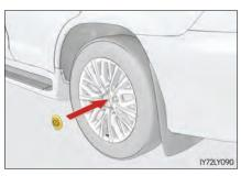
Remove the center wheel ornament from the flat tire by pushing from the reverse side, and reinstall it.
