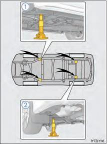
6 Raise the vehicle until the tire is slightly raised off the ground.
