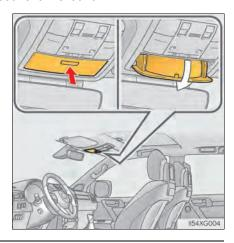
To use the overhead console when the conversation mirror is open, further extend the lid.  $(\rightarrow P.~400)$
