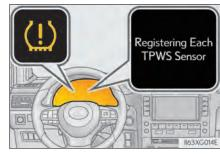
When registration is being performed, the tire pressure warning light will blink for approximately 1 minute then illuminate and "--" will be displayed for the inflation pressure of each tire on the multi-information display.
