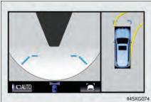
• When checking the area to the sides of the vehicle (side views)
