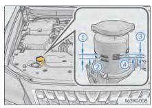
Hot: The vehicles has been driven around 50 mph (80 km/h) for 20 minutes, or slightly longer in frigid temperatures. (Fluid temperature,  $140^{\circ}F - 175^{\circ}F [60^{\circ}C - 80^{\circ}C]$ ).
