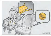
Seat belts equipped with a child restraint locking mechanism (ALR/ ELR belts except driver's seat belt)  $(\rightarrow P.32)$
