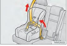
6 If the child restraint has a top tether strap, the top tether strap should be latched onto the top tether strap anchor. (→P. 66)
