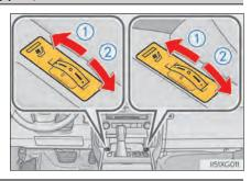
The seat heaters and ventilators can be used when the engine switch is in IGNITION ON mode.
