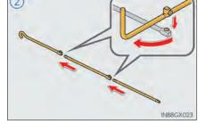
3 Assemble the jack handle extension bar and the jack handle and tighten the screw.
