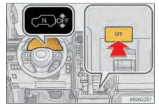
When vehicle speed exceeds 18 mph (30 km/h), the rear height control air suspension turns on automatically.
