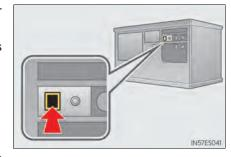
Press and hold the desired HomeLink<sup>®</sup> button (inside the vehicle) for 2 seconds and release it. Repeat this sequence (press/hold/release) up to 3 times to complete programming. If the garage door opener motor operates when the HomeLink<sup>®</sup> button is pressed, the garage
