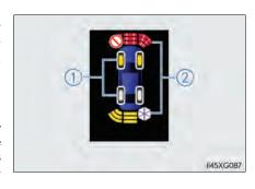
2 Pop-up display of the intuitive parking assist Displayed if an obstacle is detected while the intuitive parking assist is turned on.
