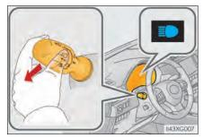
Press the Automatic High Beam switch.
