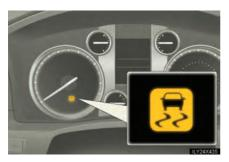
The slip indicator light flashes to indicate that the VSC/Trailer Sway Control/Active TRAC/hill-start assist control systems have been engaged.
