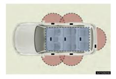
When locking or unlocking the doors
