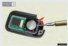
Remove the depleted battery.
