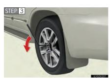
Slightly loosen the wheel nuts (one turn).
