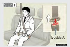
Push the release button on buckle A
