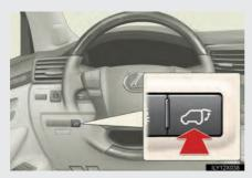
The power back door can be opened/closed using the power back door switch or wireless remote control.  $(\rightarrow P. 48)$
