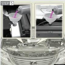
The coolant level is satisfactory if it is between the "F" and "L" lines on the reservoir.
