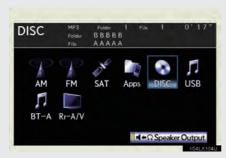
Select disc mode on the source screen to display the control screen.
