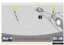
STEP 5 Turn the steering wheel with the vehicle stopped until the blue outline meets the desired parking space.
