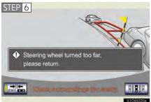
Keep the steering wheel in its current position and backing up.
