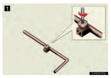
**1** Loosen the screw using a screwdriver.
