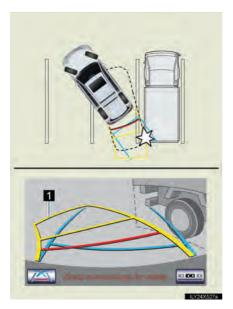
Visually check the surroundings and the area behind the vehicle. In the case shown in the illustration, the truck appears to be outside of the estimated course lines and the vehicle does not look as if it hits the truck. However, the rear body of the truck may actually cross over the estimated course lines. In reality if you back up as guided by the estimated course lines, the vehicle may hit the truck.
