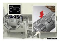
When the height control OFF switch is pressed with the vehicle stopped.
