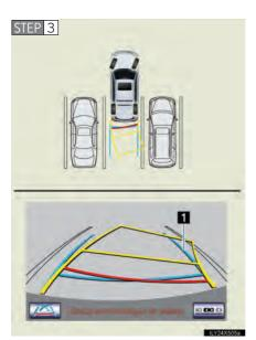
When the rear position of the vehicle has entered the parking space, turn the steering wheel so that the vehicle width extension guide lines are within the left and right dividing lines of the parking space.
