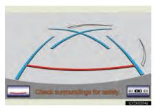
The steering wheel return points (parking assist guide lines) are displayed.
