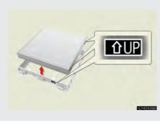
Remove the air conditioning filter and replace it with a new one.
