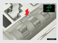
Press the Turn Assist switch while Crawl Control is operating.
