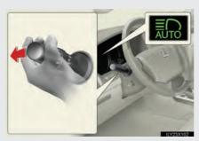
Push the lever away from you with the headlight switch in the "AUTO" position when the "ENGINE START STOP" switch is in IGNI-TION ON mode.
