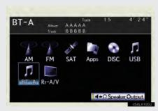
Select BT-A mode on the source screen to display the control screen.
