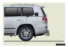
1 Hitch receiver pin hole position: 45.3 in. (1151 mm)
