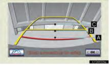
Visually check the surroundings and the area behind the vehicle. On the screen, it appears that a truck is parking at point B. However, in reality if you back up to point A, you will hit the truck. On the screen, it appears that A is closest and C is furthest away. However, in reality, the distance to A and C is the same, and B is farther than A and C.
