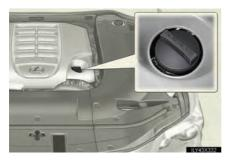
If the oil level is below or near the low level mark, add engine oil of the same type as already in the engine.  $(\rightarrow P. 885)$
