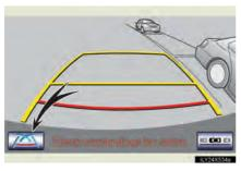
Each time you touch the display mode switch screen button, the display mode switches in the following order:
