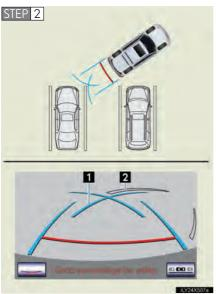
Back up until the parking assist guide line meets the edge of the left-hand dividing line of the parking space.
