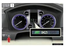
While the odometer is being displayed, press and hold the odometer/trip meter display change button to display the Eco Driving Indicator Light customization screen.
