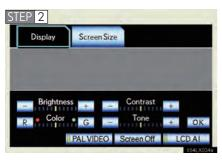
Turn "PAL VIDEO" on when PAL format equipment is connected to the A/V input port.
