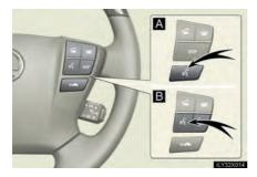
/ to operate Press or the voice command system. (→P. 429/"Navigation System Owner's Manual")
