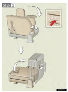
If the switch is pressed and held, the seat will automatically fold and lift sideward. (The buzzer sounds twice when the seat is about to lift.)
