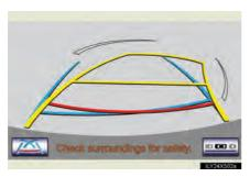
Estimated course lines are displayed which move in accordance with the operation of the steering wheel.
