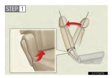
Fold the seatback while pulling the seatback angle lever. Return the seatback and secure it at the first lock position.  $(\rightarrow P. 71)$
