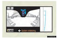
If the battery is disconnected and connected again, the message "System initializing" will be displayed on the screen. The help screen appears when "?" is touched. Make a correction using the following method in accordance with the display.
