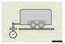
The load placed on the trailer hitch ball.  $(\rightarrow P. 385)$
