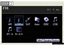
Press the "SOURCE", button to display the audio source selection screen.
