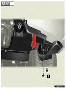
Remove the fender liner bolts, loose the fender liner nut and pull down the fender liner.
