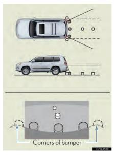
The rear view monitor system displays an image of the view from the bumper of the rear area of the vehicle.
