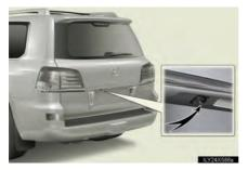
The camera for the parking assist monitor is located above the license plate.
