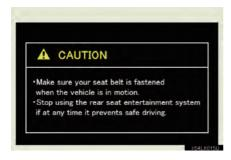
This screen appears for a few seconds when the "ENGINE START STOP" switch is in ACCESSORY or IGNITION ON mode.
