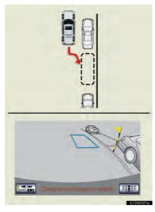
Screen display and beep sounds provide an estimation of the point at which you should turn the steering wheel when parallel parking. If the position the vehicle is to be parked in is narrower than usual, narrow mode can be used.
