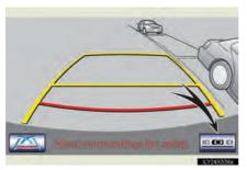
Each time you touch the parking mode switch screen button, the perpendicular parking mode and parallel parking mode are switched.
