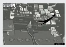
Remove the fuse with the pullout tool.
