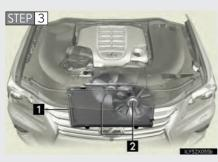
After the engine has cooled down sufficiently, inspect the radiator core (radiator) for any leaks.
