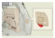
Pull the seat lock release lever and lower the seat, then lock the seat leg lock to the floor.
