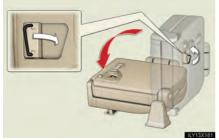
The seatback striker will be automatically stowed when the seat is lowered.
