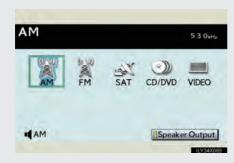
Select radio mode on the source screen to display the control screen.
