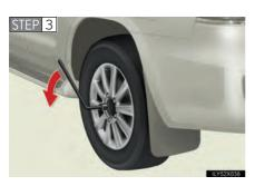
Slightly loosen the wheel nuts (one turn).
