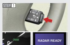
Press the "ON-OFF" button to activate the cruise control.
