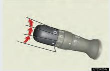
The side marker, parking, tail, license plate, daytime running lights and instrument panel lights turn on.
