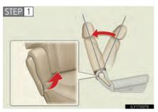
Fold the seatback while pulling the seatback angle lever. Return the seatback and secure it at the first lock position.  $(\rightarrow P. 66)$
