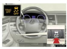
Push and hold the button for more than 3 seconds while the vehicle is stopped to turn off Active TRAC and VSC.
