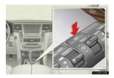
Push while the vehicle is stopped. The "OFF" indicator will appear on the multi-information display, and the vehicle height will be fixed in the current mode. Push the switch again to turn the system back on.
