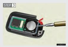
Remove the depleted battery.
