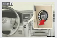
Press the "ENGINE START STOP" switch.
