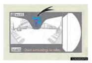
If the wide view front & side monitor is switched to from the Lexus parking assist monitor, the icon display area will flash to inform the driver that the currently displayed area is the front or side. The icon display area will continue to flash until the screen is turned off.
