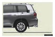
Hitch receiver pin hole position: 45.3 in. (1151 mm)
