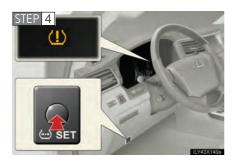
Push and hold the tire pressure warning reset switch until the tire pressure warning light blinks slowly 3 times and a message appears on the multi-information display.
