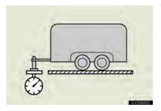
The load placed on the trailer hitch ball.  $(\rightarrow P. 303)$
