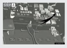
Remove the fuse with the pullout tool.
