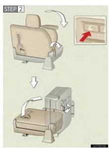
If the switch is pressed, the seat will automatically fold and lift sideward.
