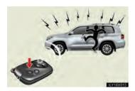
When it is pressed for longer than about one second, the head lights/tail lights/emergency flashers will flash, the front and rear interior lights will come on, and an alarm will sound for about 60 seconds to deter any person from trying to break into or damage your vehicle.
