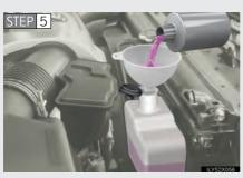
Add engine coolant if necessary.
