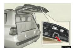
Pressing the switch closes upper back door automatically. (A buzzer sounds)
