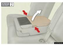
Press the button to release the lock.
