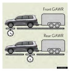
The maximum allowable gross axle weight. The gross axle weight is the load placed on each axle (front and rear).
