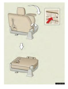
The seat will automatically fold when the switch is pressed.
