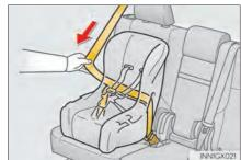
Shill pushing the child restraint system into the seat, allow the shoulder belt to retract until the child restraint system is securely in place.
