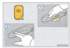
2 Touch the lock sensor (the indentation on the upper part or lower part of the front door handle) to lock the doors.
