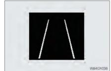
When solid lane lines are shown: The LDA system is active.
