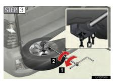
Insert the jack handle extension into the lowering socket.
