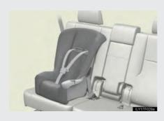
Seat belts equipped with a child restraint locking mechanism (ALR/ELR belts except driver's seat belt) (→P. 88)
