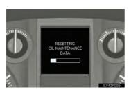
The message shown in the illustration will appear on the display. After 5 seconds, the system reset will be completed.
