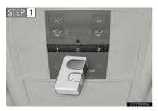
Point the remote control transmitter for the device 1 in. (25 mm) from the HomeLink $^{\textcircled{R}}$  buttons.
