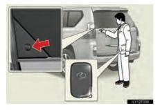
Press the button to open the glass hatch. The glass hatch will pop up.
