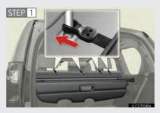
Attach the hooks to the head restraints.
