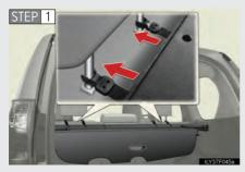
Attach the hooks to the head restraints.
