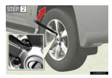
Pry off the wheel ornament, using the beveled end of the wheel ornament remover as shown.
