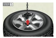
Pull out the spare tire and remove the holding bracket.
