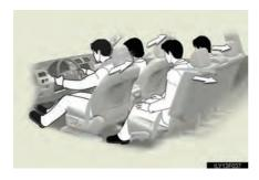
The pretensioner helps the seat belt to quickly restrain the occupant by retracting the seat belt when the vehicle is subjected to certain types of severe frontal collision or side collision.
