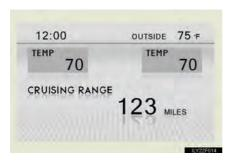
Displays the estimated maximum distance that can be driven with the quantity of fuel remaining
