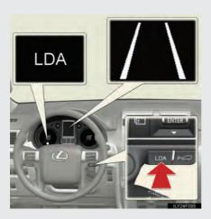
Press the "LDA" switch to activate the system.
