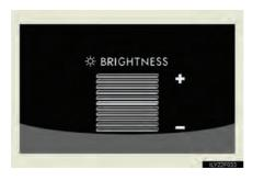
Press the display adjustment switch (" $\land$ " or " $\lor$ ") to adjust the brightness.
