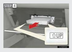
Replace the filter with a new one.
