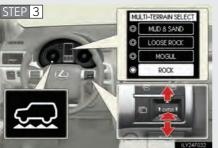
Press the "ENTER" switch upwards or downwards to select a desired mode and then press the "ENTER" switch.
