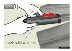
Push the case while pressing the lock release button.
