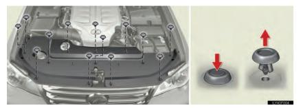
■ Installing the clips
