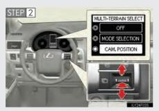
Move the "ENTER" switch upwards or downwards to select "CAM. POSITION", and press the "ENTER" switch.
