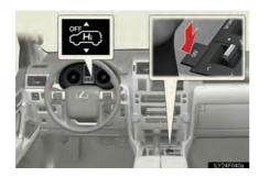
When the height control OFF switch is pressed with the vehicle stopped, the vehicle height is fixed at the current height.
