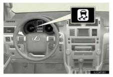
If the vehicle is in danger of slipping or rolling backward when starting on an incline, or if any of the drive wheels spins, the slip indicator light flashes to indicate that the VSC/TRAC or Active TRAC/hill-start assist control systems are operating.
