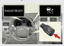
Selecting vehicle-to-vehicle distance control mode:
