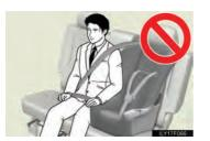
When using the left side LATCH anchors for the child restraint system, do not sit in the center seat.
