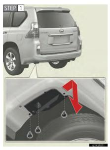
Remove the bolts and pull down the under cover.
