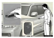
Touch the lock sensor (the indentation on the upper or lower part of the door handle) to lock the doors.
