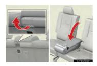
Pull the center seatback lock release lever behind the seatback and fold it down.
