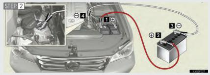
Connecting the jumper cables according to the following procedure:
