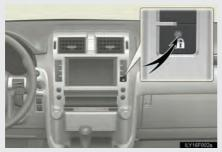
Close the doors, glass hatch and hood, and lock all the doors. The system will be set automatically after 30 seconds.
