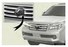
The radar sensor detects vehicles or other obstacles on or near the road ahead and determines whether a collision is imminent based on the position, speed, and heading of the obstacles.
