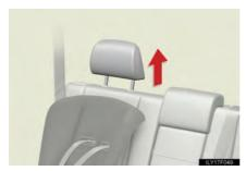
Move the head restraint in place at the upmost position.
