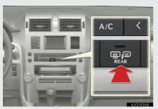
Turns the rear window and outside rear view mirror defoggers on/off.
