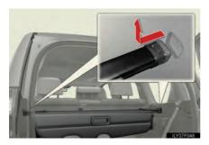
Retract the cover and release both ends, then lift it out.
