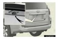
The rear view monitor camera is located on the back door as shown in the illustration. The camera uses a special lens. The distance of the image that appears on the screen differs from the actual distance.
