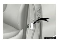
For the GAWR, see the Certification Label. For the maximum load of the tire, see the load limit at maximum cold tire inflation pressure mentioned on the sidewall of the tire.  $(\rightarrow P, 767)$
