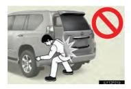
• The back door may close if the back door stopper is not locked (specifically, when using the luggage compartment with the back door kept open at your desired position). It is more difficult to open or close the back door on an incline than on a level surface, so beware of the back door unexpectedly opening or closing by itself. Make sure that the back door stopper is locked and secure when using the luggage compartment.
