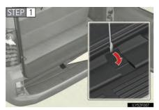
Remove the spare tire carrier lid using a flathead screwdriver.
