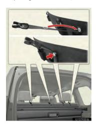
Fasten the button when the second seats are in the rear-most position.
