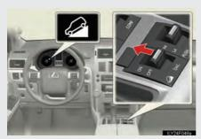
Shift the "DAC" switch to ON. The downhill assist control indicator light comes on and the system will operate.
