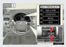
Press the "ENTER" switch upwards or downwards until "MULTI-TERRAIN SELECT" appears and then press the "ENTER" switch.
