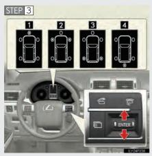
The camera view can be switched by moving the "ENTER" switch upwards or downwards.
