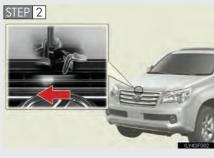
Move the auxiliary catch lever to side direction and lift the hood.
