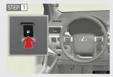
Press the opener to open the fuel filler door.
