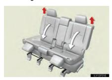
Pull the seatback lock release lever and fold them down.
