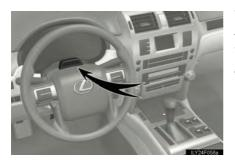
The driver monitor sensor detects the direction the driver is facing. The system determines whether the driver is facing forward.
