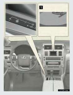
The rear view image is displayed when the shift lever is in the R position.
