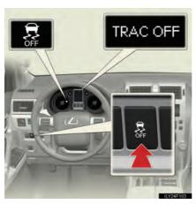
To turn the TRAC or Active TRAC and VSC systems off, press and hold the button for more than 3 seconds while the vehicle is stopped.
