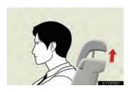
Always raise the head restraint one level from the stowed position when using.
