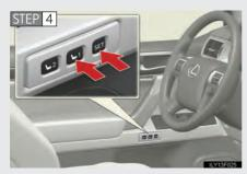
While pressing the "SET" button, or within 3 seconds after the "SET" button is pressed, press button 1 or 2 until the signal beeps.
