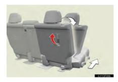
Pull the release lever and fold down the seatback. The seat will slide forward.
