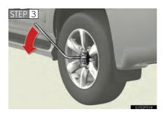
Slightly loosen the wheel nuts (one turn).
