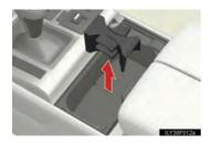
Cup holder insert may be removed for cleaning.
