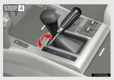
Pry the cover up with a flathead screwdriver or tool.
