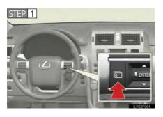
Press and hold the menu switch to display customization mode.
