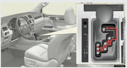
While the "ENGINE START STOP" switch is in IGNITION ON mode, move the shift lever with the brake pedal depressed.
