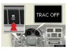
To turn the TRAC or Active TRAC system off, quickly press and release the button.
