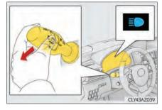
**2** Press the Automatic High Beam switch.
