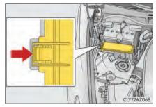
► Engine compartment (type B fuse box)
