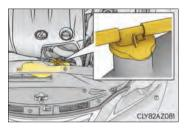
IS200t: Do not loosen the coolant reservoir cap or intercooler reservoir cap while the engine and radiator are hot.
