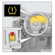
Wait for a few minutes with the engine switch in IGNITION ON mode and then turn the engine switch off.
