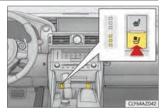
The seat ventilators can be used when the engine switch is in IGNITION ON mode.
