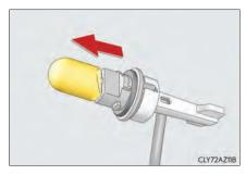
for Install a new light bulb then install the bulb base to the light unit by inserting it and turning the bulb base clockwise.
