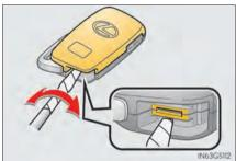
Remove the depleted battery.
