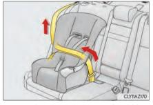
If the child restraint has a top tether strap, the top tether strap should be latched onto the top tether strap anchor.  $(\rightarrow P. 65)$
