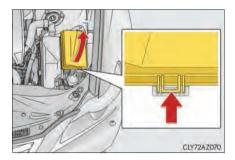
Driver's side instrument panel Remove the lid.
