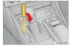
**5** Press the shift lock override button. The shift lever can be shifted while the button is pressed.
