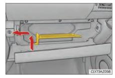
3 Press the tabs and remove the filter cover.
