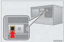
6 Press and hold the programmed HomeLink® button (located inside the vehicle) for 2 seconds and release it. Repeat this sequence (press/hold/release) up to 3 times to complete programming.
