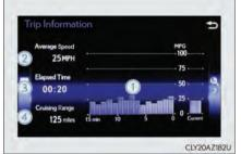
Average fuel consumption for the past 15 minutes is divided by color into past averages and averages attained since the engine switch was last turned to IGNITION ON mode. Use the displayed average fuel consumption as a reference.
