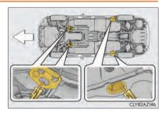
If you use chains or cables to tie down your vehicle, the angles shaded in black must be  $45^{\circ}$ .
