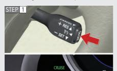
Press the "ON-OFF" button to activate the cruise control.
