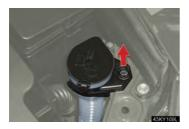
Remove the securing bolt and move the washer fluid filler opening to allow easy access to the light bulbs.
