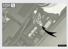
Remove the fuse with the pullout tool.
