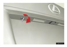
Turn the mechanical key clockwise to open.
