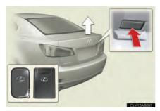
Press the button to unlock the trunk.
