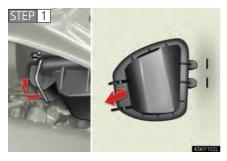
Release the lock and remove the cover.
