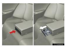
To open, press in and release the rear cup holder on the rear center armrest.
