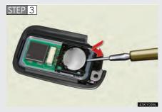
Remove the depleted battery.
