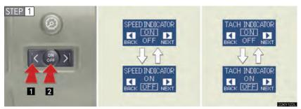
Push "<" or ">" to select the speed or tacho indicator set mode. (11) Turn the speed or tacho indicator to "OFF" and then "ON" by pushing the "ON/OFF" button. (12)
