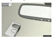
Point the remote control transmitter for the device 1 to 3 in. (25 to 75 mm) from the HomeLink  $^{\$}$  buttons.
