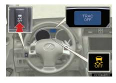
Push and hold the switch for more than 3 seconds or more while the vehicle is stopped to turn off TRAC and VSC.
