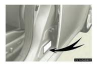
For the GAWR, see the Certification Label. For the maximum load of the tire, see the load limit at maximum cold tire inflation pressure mentioned on the sidewall of the tire.  $(\rightarrow P. 530)$
