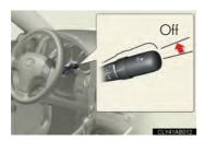
Set the wiper switch to off. If the wiper switch is in "AUTO", the wipers may operate unexpectedly in the following situations, and may result in hands being caught or other serious injuries and cause damage to the wiper blades.
