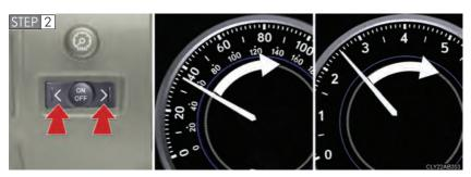
Push "<" or ">" within 6 seconds of the speedometer or tachometer needle moving to change the setting of the desired speed, then turn the indicator mode to "ON" by pushing the "ON/OFF" button.
