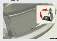
Pull the lever upwards when lifting the luggage mat up.
