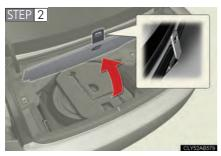
Secure the panel using the hook provided.
