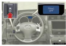
Quickly push and release the switch to turn off TRAC.
