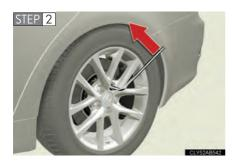
Slightly loosen the wheel nuts (one turn).
