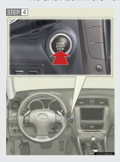
Press the "ENGINE START STOP" switch.
