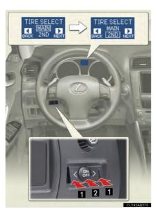
Tire pressure warning valve and transmitter ID code settings display
