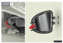
Release the lock and remove the cover.
