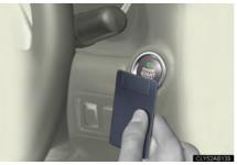
Touch the Lexus emblem side of the electronic key to the "FNGINE START STOP" switch.
