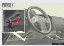
Hold the steering wheel and press the lever down.
