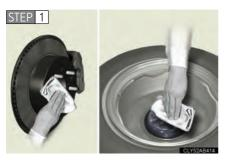
Remove any dirt or foreign matter from the wheel contact surface.
