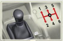
Fully depress the clutch pedal before operating the shift lever, and then release it slowly.
