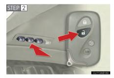
While the desired button ("1", "2" or "3") press on the wireless remote control until the signal beeps.
