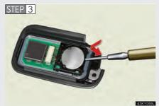
Remove the depleted battery.
