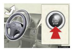
When the "ENGINE START STOP" switch is turned OFF, the steering wheel returns to its stowed position by moving up and away to enable easier driver entry and exit.
