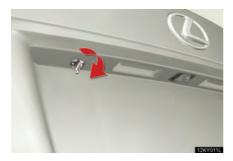
Turn the mechanical key clockwise to open.
