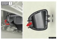
Release the lock and remove the cover.
