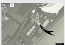
Remove the fuse with the pullout tool.
