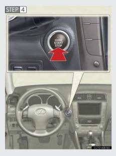
Press the "ENGINE START STOP" switch.
