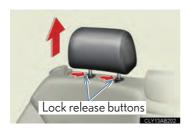
Pull the head restraint up while pushing both of the lock release buttons.
