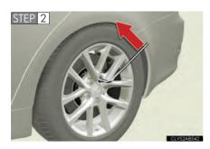
Slightly loosen the wheel nuts (one turn).
