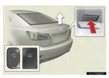
Press the button to unlock the trunk.
