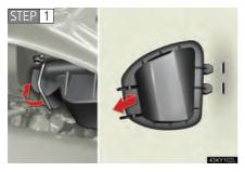
Release the lock and remove the cover.
