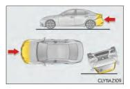
The SRS curtain shield airbags do not generally inflate if the vehicle is involved in a rear collision, if it rolls over, or if it is involved in a low-speed side or low-speed frontal collision.
