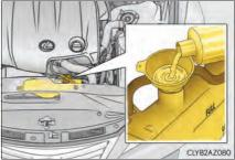
6 Start the engine and turn the air conditioning system on to check that the radiator cooling fan operates and to check for coolant leaks from the radiator or hoses.
