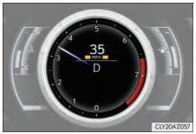
The indicator will illuminate in yellow at an optionally set speed and red at the fixed high speed.
