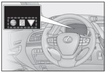
When a tab other than the Driving support system information display is selected, only a recognized speed limit sign or do not enter sign (when notification is necessary) will be displayed. (→P.90)
