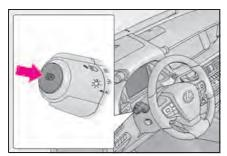
2 Push the lever away from you with the headlight switch in the **■**○ or AUTO position.
