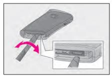
3 Remove the depleted battery.
