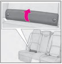
3 Insert the tab **B** into the slit **A** of the cover.
