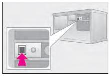
3 Press and hold the desired HomeLink® button (inside the vehicle) for 2 seconds and release it. Repeat this sequence (press/hold/release) up to 3 times to complete programming. If the garage door opener motor operates when the HomeLink® button is pressed, the garage door
