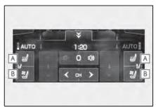
Adjust the rear seat heater temperature level
