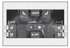
Adjust the rear seat heater temperature level
