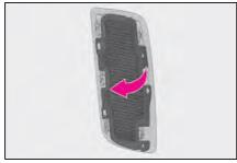
3 Remove any dust and clogs from the filter using a vacuum cleaner, etc.
