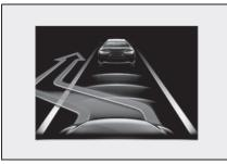
Indicates that steering wheel assist of the lane change assist function is operating.
