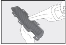
4 Install the filter in its original position, and then install the grille.
