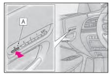
2 Using the seat adjustment switches on the driver's seat, adjust the front passenger's seat.
