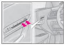
To record the position of the front passenger's seat, adjust the front passenger's seat to the desired position and perform step 4 using the buttons on the front passenger's side.
