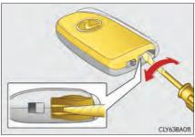
Remove the depleted battery.
