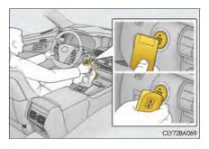
3 Press the engine switch within 10 seconds of the buzzer sounding, keeping the brake pedal depressed.
