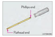
**3** Using the flathead end of the screwdriver, remove the clips.
