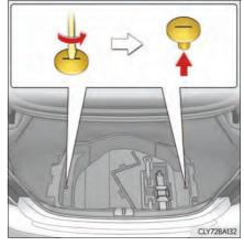
4 While lifting the rear side of the left and right side deck boards, remove the tool tray.
