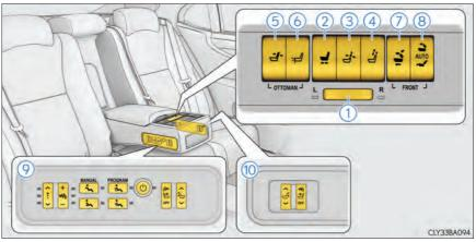
The right-hand rear seat is a relaxation seat, which is equipped with a seatback angle adjustment function and an ottoman.
