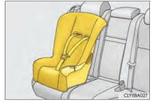
Run the seat belt through the child restraint system and insert the plate into the buckle.
