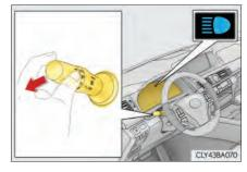
**2** Press the Automatic High Beam switch.
