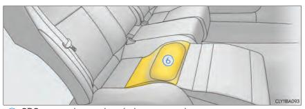
SRS seat cushion airbag (relaxation seat)Can help restrain the relaxation seat occupant
