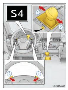
The initial shift range in S mode is set automatically between 3 and 7 according to vehicle speed and driving conditions.
