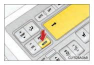
The rear controller can be locked from the air conditioning operation screen.  $(\rightarrow P.348)$
