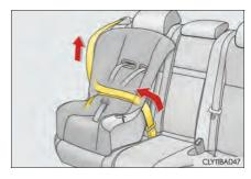
If the child restraint has a top tether strap, the top tether strap should be latched onto the top tether strap anchor.  $(\rightarrow P. 74)$
