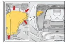
► Engine compartment (type B fuse box)
