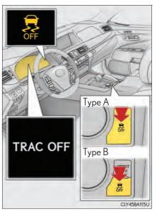
\*: On vehicles with pre-collision system, pre-collision alert braking, pre-collision brake assist and pre-collision braking will also be disabled. The pre-collision system warning light will come on and the "Pre-collision brakes are disabled because VSC is OFF" will be shown on the multi-information display. (\$\rightarrow\$P. 295)
