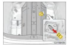
6 Replace the screwdriver head with the parking brake release tool.
