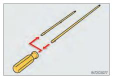
Insert the tool and press it down firmly while turning it counterclockwise until it stops.
