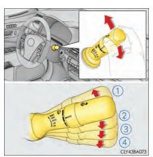
When "AUTO" mode is selected, the sensor sensitivity can be adjusted by turning the switch ring.
