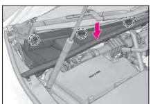
**2** Engage the rubber strip to the vehicle body.
