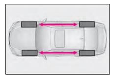
To equalize tire wear and extend tire life, Lexus recommends that tire rotation is carried out at the same interval as tire inspection.
