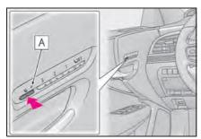
2 Using the seat adjustment switches on the driver's seat, adjust the front passenger's seat.
