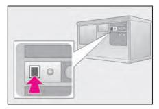
3 Press and hold the desired HomeLink® button (inside the vehicle) for 2 seconds and release it. Repeat this sequence (press/hold/release) up to 3 times to complete programming. If the garage door opener motor operates when the HomeLink® button is pressed, the garage door opener motor recognizes the HomeLink® signal.
