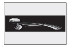
The curve display on the head-up display changes according to the direction and curvature of the curve.
