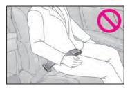
The SRS front passenger airbag also deploys with considerable force, and can cause death or serious injury especially if the front passenger is very close to the airbag. The front passenger seat should be as far from the airbag as possible with the seatback adjusted, so the front passenger sits upright.
