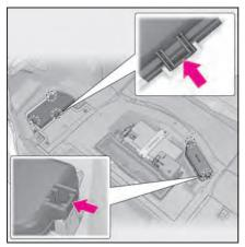
3 Remove the fuse with the pullout tool.
