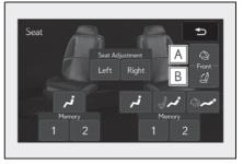
A Move the front passenger's seat forward and fold the seatback forward.
