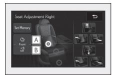
A Touch and hold to move the front passenger's seat forward and fold the seatback forward.
