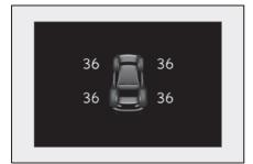
If the tire pressure drops below a predetermined level, the driver is warned by a screen display and a warning light. (→P.422)
