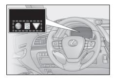
When a tab other than the driving support system information tab is selected, only a recognized speed limit sign or do not enter sign (when notification is necessary) will be displayed. (→P.76)
