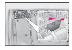
6 Connect a positive jumper cable clamp to A on your vehicle and connect the clamp on the other end of the positive cable to B on the second vehicle. Then,
