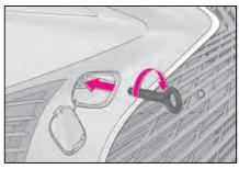
4 Tighten down the towing eyelet securely using a phillips-head screwdriver or hard metal bar.
