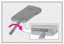
3 Remove the depleted battery.
