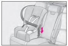
4 Fully extend the shoulder belt and allow it to retract to put it in lock
