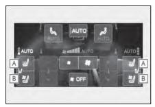
Adjust the rear seat heater temperature level
