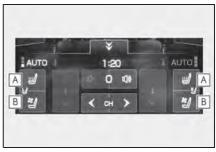
A djust the rear seat heater temperature level
