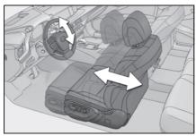
On vehicles with adjustable seat cushion side bolsters, when the driver's door is opened with the engine switch off, the seat cushion side bolsters will lower if they are in the default position.
