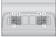
A Increases the rear seat heater temperature level
