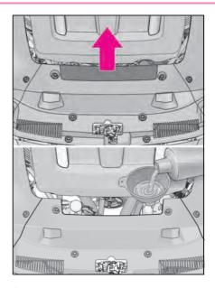
Start the engine and turn the air conditioning system on to check that the radiator cooling fan operates and to check for coolant leaks from the radiator or hoses.
