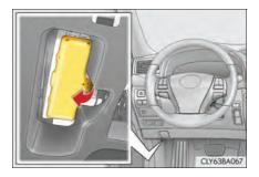
▶ Passenger's side instrument panel Remove the lid.
