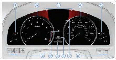
The units used on the speedometer and the tachometer may differ depending on the target region.
