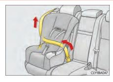
If the child restraint has a top tether strap, the top tether strap should be latched onto the top tether strap anchor.  $(\rightarrow P. 72)$
