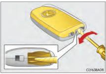
Remove the depleted battery.
