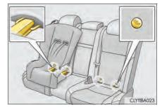
Seat belts equipped with a child restraint locking mechanism (ALR/ELR belts except driver's seat belt) ( $\rightarrow$ P. 38)
