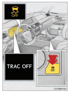
\*: On vehicles with pre-collision system, pre-collision alert braking, pre-collision brake assist and pre-collision braking will also be disabled. The pre-collision system warning light will come on and the "Pre-collision brakes are disabled because VSC is OFF" will be shown on the multi-information display. (→P. 296)
