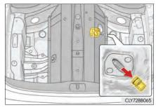
Replace the screwdriver head with the parking brake release tool.
