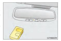
Press and hold one of the HomeLink<sup>®</sup> buttons and the transmitter button. When the HomeLink<sup>®</sup> indicator light changes from a slow to a rapid flash, you can release both buttons.
