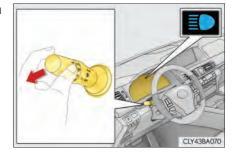
**2** Press the Automatic High Beam switch.
