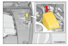
► Engine compartment (type C fuse box)
