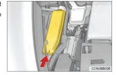
► Engine compartment (type B fuse box)
