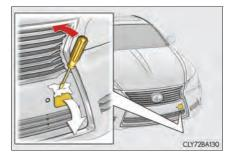
3 Insert the towing eyelet into the hole and tighten partially by hand.
