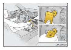
3 Press the power switch within 10 seconds of the buzzer sounding, keeping the brake pedal depressed.
