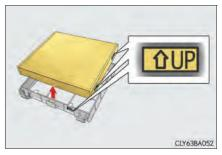
**7** Reset the air conditioning filter maintenance data.  $(\rightarrow P. 477)$
