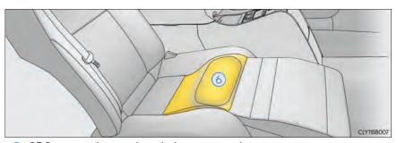
SRS seat cushion airbag (relaxation seat)Can help restrain the relaxation seat occupant
