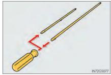
Insert the tool and press it down firmly while turning it counter-clockwise until it stops.
