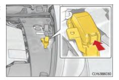
▶ Engine compartment (fuse box near the power control unit)
