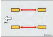
To equalize tire wear and extend tire life, Lexus recommends that tire rotation is carried out at the same interval as tire inspection.
