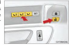
To prevent unintended triggering of the alarm, open and close a door once after a driving position has been recorded. (If a door is not opened within 30 seconds after is pressed, the doors will be locked again and the alarm will automatically be set.)
