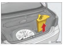
**3** Remove the jack after removing the hook.
