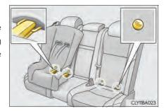
Seat belts equipped with a child restraint locking mechanism (ALR/ELR belts except driver's seat belt) (→P. 40)
