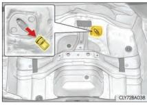
5 Insert the tool and press it down firmly while turning it counterclockwise until it stops.
