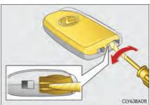
Remove the depleted battery.
