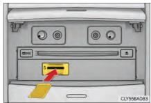
Insert the SD card with the label side up, positioning the cut off corner to the right. When it is inserted, push it straight in until you hear a click.
