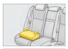
2 Sit the child in the child restraint system. Fit the seat belt to the child restraint system according to the manufacturer's instructions and insert the plate into the buckle. Make sure that the belt is not twisted.
