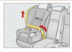
**5** If the child restraint has a top tether strap, the top tether strap should be latched onto the top tether strap anchor.  $(\rightarrow P. 73)$
