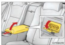
1 Open the cover and connect audio-video equipment to the A/V input port.
