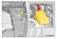
► Engine compartment (type C fuse box)
