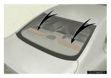
There are air intake vents on the package tray for the purpose of cooling the hybrid battery (traction battery). If the vents become blocked, the hybrid battery may overheat, leading to a reduction in hybrid battery output.
