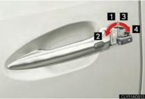
Remove the cover on the driver's door handle using the mechanical key ( $\rightarrow$ P. 48) in order to perform the following operations:
