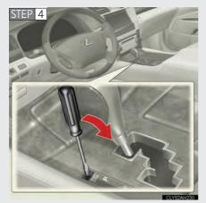
Pry the cover up with a flathead screwdriver or equivalent.
