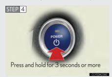
Stop the hybrid system by pressing and holding the "POWER" switch for 3 consecutive seconds or more.
