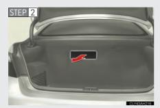
Open the trunk lid. Remove the filter cover.
