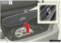
Secure the panel using the hook provided.
