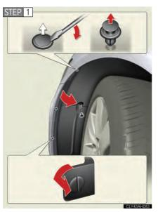
To allow enough working clearance, turn the steering wheel to the opposite side of the bulb to be replaced.
