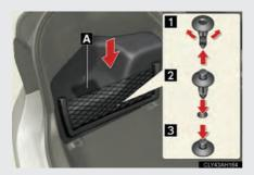
Install the 12-volt battery cover with the clip. Press down on the cover at position "A" to secure it.
