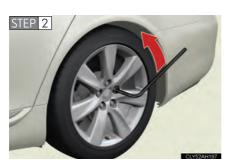
Slightly loosen the wheel nuts (one turn).
