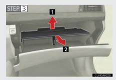
Open the glove box. Lift and remove the partition.
