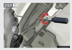
Turn bolt B the same number of turns and in the same direction as step 1 using a Phillips-head screwdriver.
