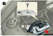
1 Remove the securing bolts and move the ECU.
