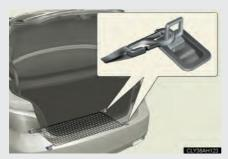
The cargo net is provided for securing loose items on the floor or items inside the trunk.
