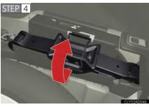
Remove the jack after removing the hook.
