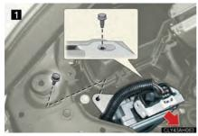
Remove the securing bolts and move the ECU.
