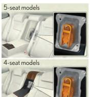
Never try to open the service plug access hole located behind the rear seat. The service plug is used only when the vehicle is serviced and is subject to high voltage.
