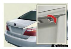
Turn the mechanical key clockwise to open.
