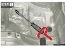
Insert the tool and press it down firmly while turning it counter-clockwise until it stops.
