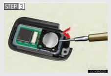
Remove the depleted battery.
