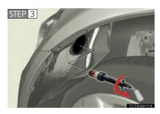
Disconnect the connector and turn the bulb socket counterclockwise.
