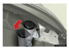
Remove the securing bolt and move the washer fluid filler opening.
