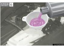
Add power control unit coolant if necessary.
