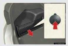
Remove the 12-volt battery cover after removing the clip.
