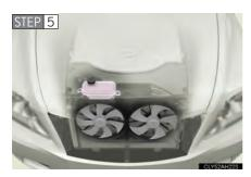
After the hybrid system has cooled down, check the engine coolant level and inspect the cooling system for leaks.
