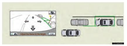
In this case, if you align the warning flag with the rear of the forward parked vehicle, and the extended green line with the lower edge of the parked vehicle's rear wheel when setting the target parking position, the left side of your vehicle will be roughly in line with the left side of the front parked vehicle once assisted parking is complete. If you are parallel parking on the opposite side of the road, left and right will be reversed.
