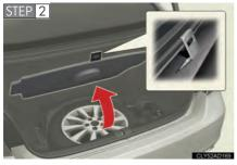
Secure the panel using the hook provided.
