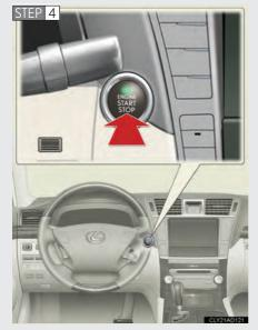
Press the "ENGINE START STOP" switch.
