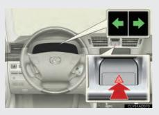
Press the switch to flash all the turn signal lights. To turn them off, press the switch once again.
