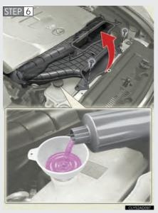
Add engine coolant if necessary.
