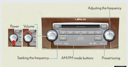
The audio control screen may differ slightly depending on the types of audio equipped.
