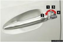
Remove the cover on the driver's door handle using the mechanical key ( $\rightarrow$ P. 33) in order to perform the following operations.
