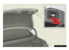
Pressing the switch closes the trunk lid automatically. (A buzzer sounds.)
