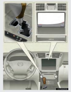
Advanced parking guidance system will activate when the shift lever is in "R" position.
