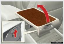
When returning the table, pull it up while pulling the lock release lever.
