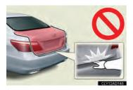
In the event that the trunk lid is left slightly open, the trunk easy closer will automatically close it to the fully closed position. It takes several seconds before the trunk easy closer begins to operate. Be careful not to catch fingers or anything else in the trunk lid, as this may cause bone fractures or other serious injuries.
