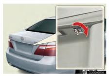
Turn the mechanical key clockwise to open.
