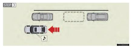
A chime will sound twice when the front edge of the vehicle parked in front of the target parking space is visible right beside you. When this chime sounds twice, stop your vehicle.
