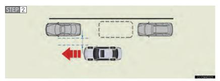
Move your vehicle slowly alongside the vehicle parked in front of the target parking space. Your vehicle should move parallel to the road or shoulder and be approximately 3 ft. (1 m) away from the side of the parked vehicle.
