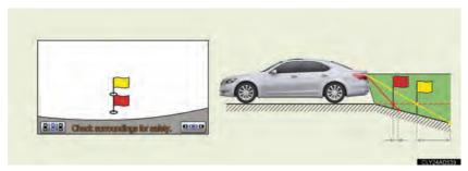
When the grade behind the vehicle slopes down sharply, objects appear to be closer than they actually are.
