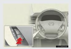
Pressing the pre-support switch while assist mode is on, the "ENGINE START STOP" switch is in IGNITION ON mode and the vehicle is traveling below 9 mph (15 km/h) with the shift position in any position other than "P" or "R", will cause the screen to change in the following order:
