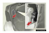
The lever can be used to open the fuel filler door if the fuel filler door cannot be opened using the inside switch.
