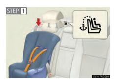
Secure the child restraint using a seat belt or a lower anchors, and move the head restraint in place at the lowest position. (→P. 89)
