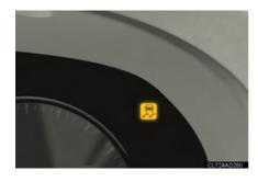
If the vehicle is in danger of slipping, rolling backwards when starting on an incline, or any of the drive wheels spin, the indicator flashes to indicate that the VSC/TRAC/hill-start assist control systems have been engaged.
