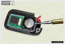
Remove the depleted battery.
