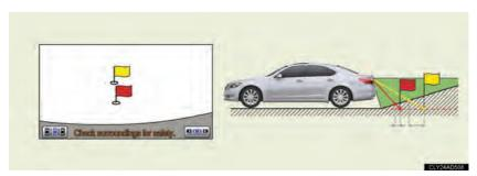
When the grade behind the vehicle slopes up sharply, objects appear to be farther away than they actually are.
