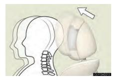
If the vehicle detects an impact during a rear-end collision, the front part of the head restraint moves forward and upward to help reduce the risk of whiplash to the seat occupant.
