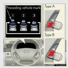
Each press of the switch changes the vehicle-to-vehicle distance
