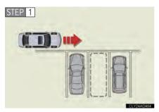
With the vehicle stopped or driving at 9 mph (15 km/h) or less, push the pre-support switch twice when your vehicle is positioned slightly before the target parking space. ( $\rightarrow$ P. 248) Check that the screen changes.
