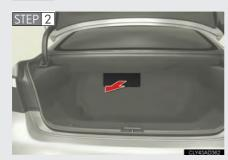
Open the trunk lid. Remove the filter cover.
