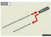
Take out the parking brake release tool and the screwdriver from the trunk.  $(\rightarrow P.720)$
