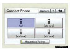
When you register your phone, auto connection will be activated. Always set it to this mode and leave the Bluetooth<sup>®</sup> phone on the place where connection can be established.
