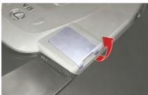
If the oil level is below or near the low level mark, add engine oil of the same type as already in the engine.
