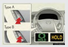
Turns the brake hold system on.
