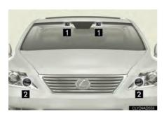
Detects pedestrians and other three-dimensional objects on or near the road ahead together with the radar sensor while the vehicle is moving. When the headlights are on, near-infrared rays are projected to ensure proper detection performance in the night time.
