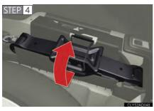
Remove the jack after removing the hook.
