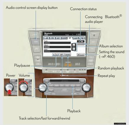
The audio control screen may differ slightly depending on the types of audio equipped.
