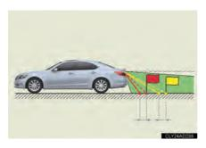
When any part of the vehicle sags due to the number of passengers or the distribution of the load, there is a margin of error between the set target parking position on the screen, and the actual distance/course on the road.
