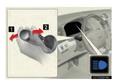
With the headlights on, push the lever away from you to turn on the high beams.
