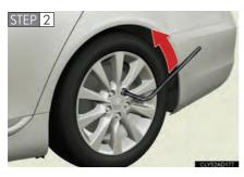
Slightly loosen the wheel nuts (one turn).
