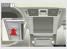
Press "CLIMATE" to display the conditioning operation screen.
