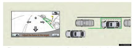
The assisted parking position will move left or right of the set target parking position.
