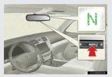
To turn the compass on or off, press and hold "AUTO" for more than 3 seconds.
