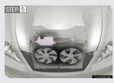
After the engine has cooled down, check the engine coolant level and inspect the cooling system for leaks.
