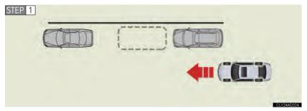
With the vehicle stopped or driving at 9 mph (15 km/h) or less, push the pre-support switch once when your vehicle is positioned slightly before the target parking space.  $(\rightarrow P. 248)$  Check that the screen changes.
