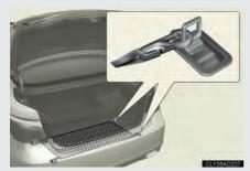
The cargo net is provided for securing loose items on the floor or items inside the trunk.
