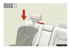
Replace the head restraint and lift it up to the uppermost lock position.
