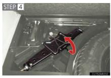
Remove the jack after removing the hook.
