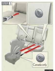
Latch the hooks of the lower straps onto the LATCH anchors. If the child restraint has a top tether strap, the top tether strap should be latched onto the top tether strap anchor bracket.
