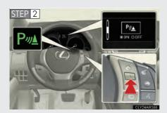
Press the "ENTER" switch to change to "ON".
