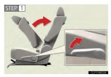
Fold the seatback while pulling the seatback angle adjustment lever. Return the seatback and secure it at the first lock position.  $(\rightarrow P. 72)$
