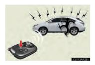
When (() is pressed for longer than about one second, an alarm will sound intermittently and the vehicle lights will flash to deter any person from trying to break into or damage your vehicle.
