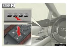
Press the desired button ("1", "2" or "3") to recall the position. Then, while keep pressing the button, press the driver's door lock switches (either lock or unlock) until the signal beeps.
