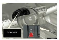
To turn the TRAC system off, quickly press and release the switch.
