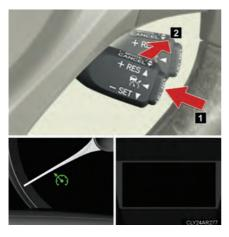
11 Press the "ON-OFF" button to activate the cruise control.
