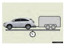
The maximum allowable gross combination weight. The gross combination weight is the sum of the total vehicle weight (including the occupants, cargo and any optional equipment installed on the vehicle) and the weight of the trailer being towed (including the cargo in the trailer).
