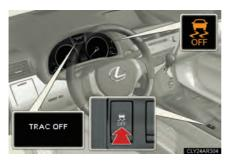
To turn the TRAC and VSC systems off, press and hold the switch for 3 seconds or more while the vehicle is stopped.
