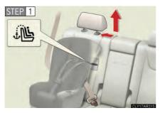
Secure the child restraint system using a seat belt or the LATCH anchors, and remove the head restraint.
