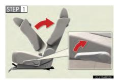
Fold the seatback while pulling the seatback angle adjustment lever. Return the seatback and secure it at the first lock position.  $(\rightarrow P. 72)$
