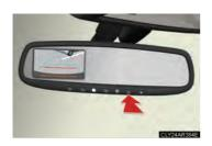
Press and hold for 12 to 15 seconds. The screen will turn off and on after 6 seconds. Keep pressing the button until the screen turns back off. The indicator will flash amber.
