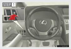
Press the opener to open the fuel filler door.
