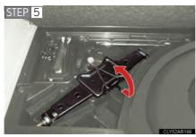
Remove the jack after removing the hook.
