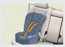
Seat belts equipped with a child restraint locking mechanism (ALR/ELR belts except driver's seat belt) (→P. 83)
