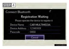
When this screen is displayed, input the passcode displayed on the screen into your Bluetooth<sup>®</sup> device.
