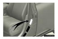
For the GAWR, see the Certification Label. For the maximum load of the tire, see the load limit at maximum cold tire inflation pressure mentioned on the sidewall of the tire. ( $\rightarrow$ P. 821)
