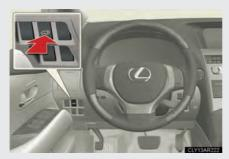
Press and hold the switch to open/close the back door.
