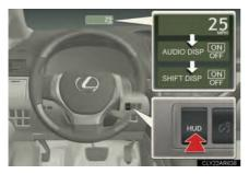
Press and hold the head-up display main switch changes the display to the display on/off mode.
