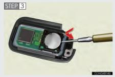
Remove the depleted battery.
