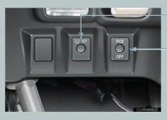
Tire pressure warning reset switch P. 686
