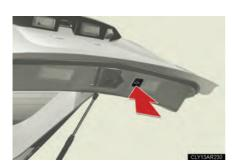
Press the switch to close the back door.
