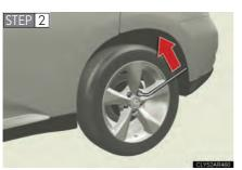
Slightly loosen the wheel nuts (one turn).
