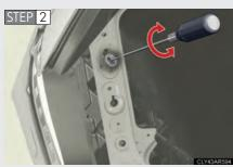
Turn bolt B the same number of turns and in the same direction as in step 1 using a Phillips-head screwdriver.
