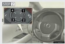
To adjust the mirror, press the switch.
