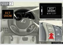
Press the "ENTER" switch to change to "ON".
