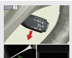
Accelerate or decelerate the vehicle to the desired speed, and push the lever down to set the speed.
