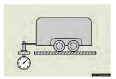
The load placed on the trailer hitch ball. ( $\rightarrow$ P. 311)
