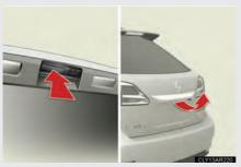
Raise the back door while pushing up the back door opener button.
