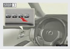
Press button "1", "2" or "3" until the signal beeps to recall the desired position.
