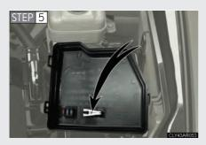
Remove the fuse with the pullout tool.
