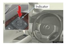
Automatic mode allows the folding or extending of the mirrors to be linked to locking/unlocking of the doors.
