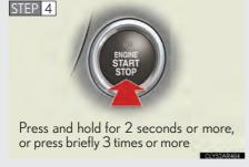
To stop the engine, press and hold the "ENGINE START STOP" switch for 2 consecutive seconds or more, or press it briefly 3 times or more in succession.
