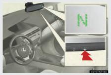
To turn the compass on or off, press for more than 3 seconds.
