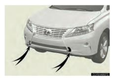
If a tow truck is not available in an emergency, your vehicle may be temporarily towed using a cable or chain secured to the emergency towing eyelet(s). This should only be attempted on hard, surfaced roads for short distances at low speeds.
