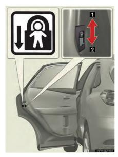
The door cannot be opened from inside the vehicle when the lock is set.
