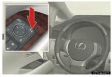
Press the switch to fold the mirrors.
