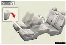
Move the seatback angle adjustment switch backward to flatten the seatback.
