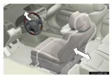
Exiting the vehicle: When all of the following actions have been performed, the steering wheel will move up and back to the point farthest away from the driver and the seat will move backward (auto away function):
