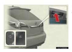
Press the button to unlock the door.
