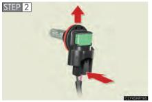
Unplug the connector while pressing the lock release.
