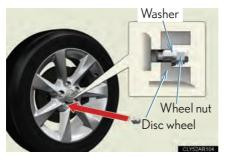
Turn the nuts until the washers come into contact with the wheel.
