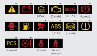
\*: These lights turn on when the "ENGINE START STOP" switch is turned to IGNITION ON mode to indicate that a system check is being performed. They will turn off after the engine is started, or after a few seconds. There may be a malfunction in a system if a light does not come on, or if the lights do not turn off. Have the vehicle inspected by your Lexus dealer, for details.
