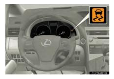
If the vehicle is in danger of slipping or rolling backward when starting on an incline, or if any of the drive wheels spins, the slip indicator light flashes to indicate that the VSC/TRAC systems are operating.
