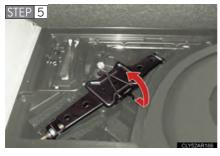
Remove the jack after removing the hook.
