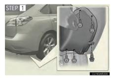
Remove the bolts using a Phillipshead screwdriver, and remove the clip.
