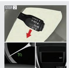
Accelerate or decelerate to the desired speed, and push the lever down to set the speed.
