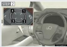
To adjust the mirror, press the switch.
