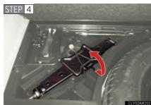
Remove the jack after removing the hook.
