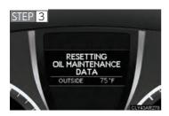
Keep the "ODO/TRIP" button pressed for about 5 seconds. The resetting procedure is complete when "00000" in the trip meter flashes once and the message in the multi-information display disappears.
