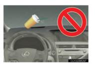
If an object falls into the opening of the headup display, remove it immediately. Also, avoid spilling water or other liquids near the headup display opening as this may cause mechanical damage.
