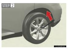
Slightly loosen the wheel nuts (one turn).
