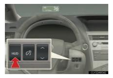
Pressing the button turns the head-up display on/off and changes the vehicle speed display units as follows:
