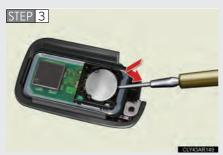
Remove the depleted battery.
