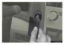
STEP 3 To change "ENGINE START STOP" switch modes: Within 10 seconds of the buzzer sounding, release the brake pedal and press the "ENGINE START STOP" switch. Modes can be changed each time the switch is pressed. (→P.150)
