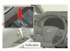
Press the switch to lock the passenger window switches.
