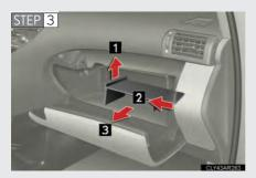
Open the glove box door. Lift and remove the partition.
