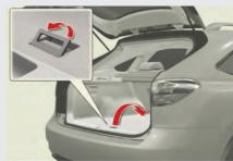
Pull the lever upwards when lifting the deck board up.
