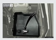
Remove the fuse with the pullout tool.
