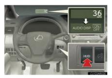
Pressing and holding the head-up display main switch button for more than 2 seconds changes the display to audio display on/off mode. Press the head-up display main switch button to turn the audio display on/off.
