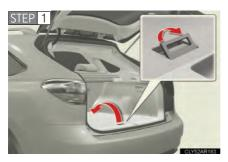
Pull the lever upward to fold back the front part of the deck board.
