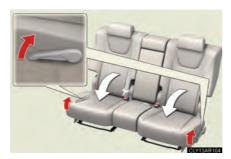
Pull the seatback angle adjustment lever.
