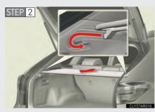
Pull out the luggage cover and hook it onto the anchors.
