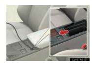
When the cover is slide open, accessory device cables can be pulled through the opening.
