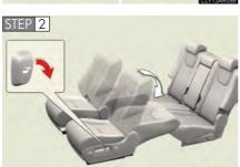
Move the front seat forward, raise the seat, and remove the head restraint  $(\rightarrow P. 72)$ .
