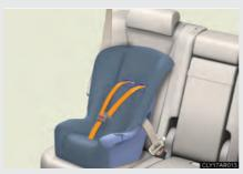
Seat belts equipped with a child restraint locking mechanism (ALR/ELR belts except driver's seat belt) (→P. 74)
