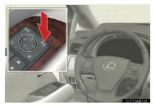
Press the switch to fold the mirrors.
