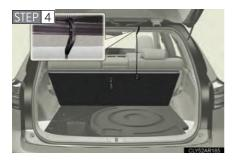
Use the hook to secure the deck board as shown in the illustration.
