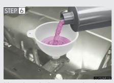
Add engine coolant if necessary.
