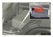
Never try to open the service plug access hole located under the rear seat. The service plug is used only when the vehicle is serviced and is subject to high voltage.
