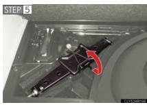
Remove the jack after removing the hook.
