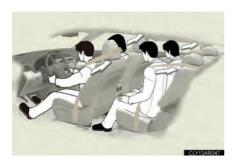
The pretensioner helps the seat belt to quickly restrain the occupant by retracting the seat belt when the vehicle is subjected to certain types of severe frontal collision.
