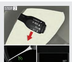
Accelerate or decelerate to the desired speed, and push the lever down to set the speed.
