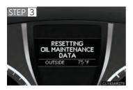
Keep the "ODO/TRIP" button pressed for about 5 seconds. The resetting procedure is complete when "000000" in the trip meter flashes once and the message in the multi-information display disappears.
