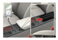
When the cover is slid open, portable audio device cables can be pulled through the opening.
