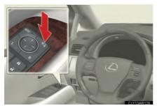
Press the switch to fold the mirrors.
