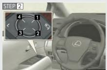
To adjust the mirror, press the switch.
