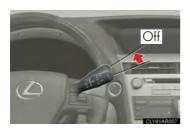
Set the wiper switch to the off position.
