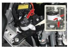
Move the washer fluid filter opening.
