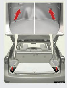
Pull the strap upwards when lifting the cover up.
