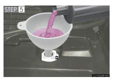
Add power control unit coolant if necessary.
