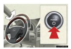
When the "POWER" switch is turned off, the steering wheel returns to its stowed position by moving up and away to enable easier driver entry and exit.
