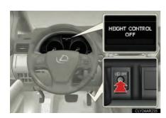
Press the height control off button while the vehicle is stopped. A message will appear on the multi-information display, and vehicle height will be fixed in the current mode.
