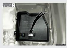
Remove the fuse with the pullout tool.
