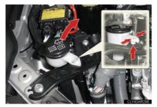
Move the washer fluid filter opening.
