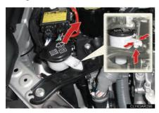
Move the washer fluid filter opening.
