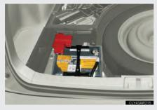
The 12-volt battery is located on the left-hand side of the luggage compartment.
