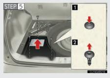
After removing the clips, remove the 12-volt battery cover.
