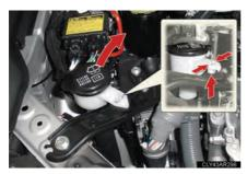
Move the washer fluid filter opening.
