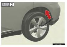
Slightly loosen the wheel nuts (one turn).
