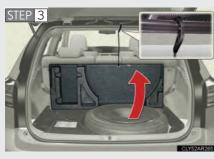
Use the hook to secure the deck board as shown in the illustration.
