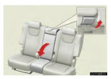
Pull the center seatback lever behind the seatback and fold the seatback down.
