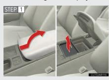
Slide the armrest while pulling up the lever, and lift the armrest. Remove the upper tray.
