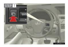
Press and hold the menu switch of the multi-information switches to display customize mode.
