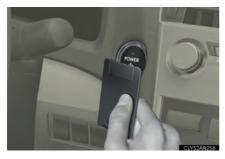
STEP 3 To change "POWER" switch modes: Within 10 seconds of the buzzer sounding, release the brake pedal and press the "POWER" switch. Modes can be changed each time the switch is pressed. (→P. 167)
