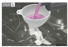
Add engine coolant if necessary.
