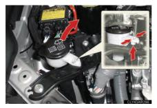
Move the washer fluid filter opening.
