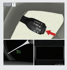
Press the "ON-OFF" button to activate the cruise control.
