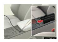
When the cover is slid open, accessory device cables can be pulled through the opening.
