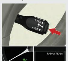
Selecting vehicle-to-vehicle distance control mode:
