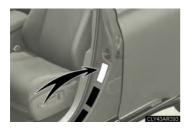
For the GAWR, see the Certification Label. For the maximum load of the tire, see the load limit at maximum cold tire inflation pressure mentioned on the sidewall of the tire.  $(\rightarrow P. 643)$
