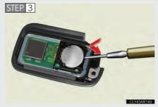
Remove the depleted battery.
