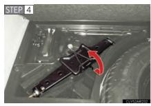
Remove the jack after removing the hook.
