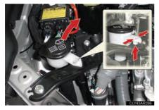
Move the washer fluid filter opening.
