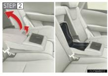
Pull up the lever to release the lock and lift the armrest.
