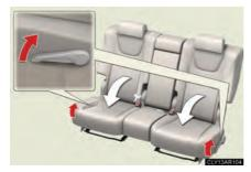
Pull the seatback angle adjustment lever.
