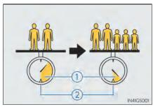
When 2 people with the combined weight of A lb. (kg) are riding in your vehicle, which has a total load capacity (vehicle capacity weight) of B lb. (kg), the available amount of cargo and luggage load capacity will be C lb. (kg) as follows:
