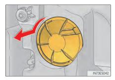
**2** Unplug the connector while pulling the lock release.
