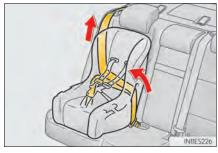
If the child restraint has a top tether strap, the top tether strap should be latched onto the top tether strap anchor.  $(\rightarrow P.63)$
