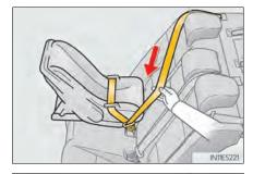
While pushing the child restraint system down into the rear seat, allow the shoulder belt to retract until the child restraint system is securely in place.
