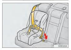
4 Fully extend the shoulder belt and allow it to retract to put it in lock mode. In lock mode, the belt cannot be extended.
