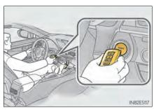
Firmly depress the brake pedal and check that is shown on the multiinformation display.
