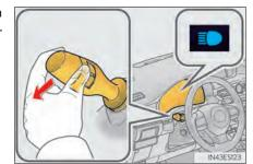
2 Press the Automatic High Beam switch.
