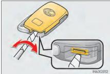
Remove the depleted battery.
