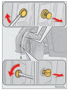
2 While holding the clamp open, pull and remove the tabs and open the fender liner.
