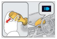
2 Press the Automatic High Beam switch.
