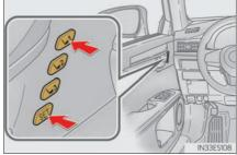
Vehicles with the driving position memory for the front passenger's seat: To record the position of the front passenger's seat, adjust the front passenger's seat to the desired position and perform step 4 using the buttons on the front passenger's side.
