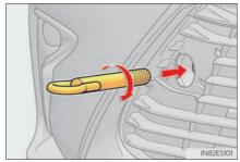
4 Tighten down the towing eyelet securely using a wheel nut wrench.
