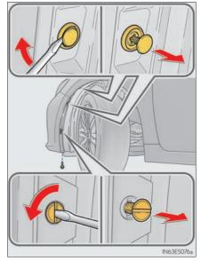
While holding the clamp open, pull and remove the tabs and open the fender liner.
