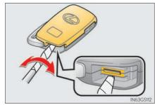
Remove the depleted battery.
