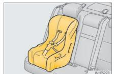
Run the seat belt through the child restraint system and insert the plate into the buckle. Make sure that the belt is not twisted.
