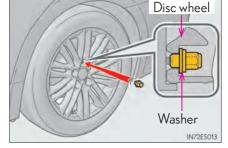
When replacing an aluminum wheel with a steel wheel, tighten the wheel nuts until the tapered portion comes into loose contact with the disc wheel seat.
