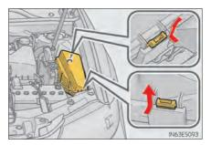
► Engine compartment (type B fuse box) (hybrid vehicles only)
