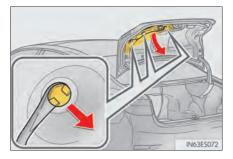
**4** Turn the bulb base counter-clockwise.
