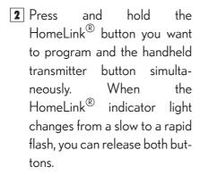
Programming has completed when the indicator light changes to a rapid flash.
