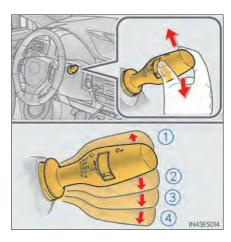
The sensor sensitivity can be adjusted when AUTO is selected.
