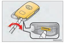
Remove the depleted battery.
