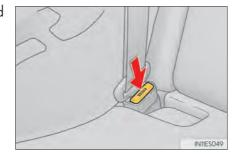
1 Lower the head restraint in place at the lowest position.
