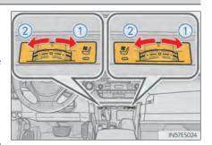
The seat heaters and ventilators can be used when the "START STOP ENGINE" <"POWER"> switch is in IGNITION ON <ON> mode.
