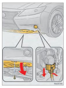
**2** Turn the bulb base counter-clockwise.
