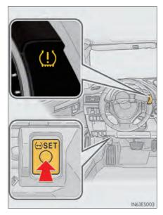
Wait for a few minutes with the "START STOP ENGINE" <"POWER"> switch in IGNITION ON <ON> mode and then turn the "START STOP ENGINE" <"POWER"> switch off.
