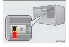
General Press and hold the programmed HomeLink® button (located inside the vehicle) for 2 seconds and release it. Repeat this sequence (press/hold/release) up to 3 times to complete programming.
