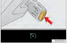
2 Accelerate or decelerate the vehicle to the desired speed, and push the lever down to set the speed.
