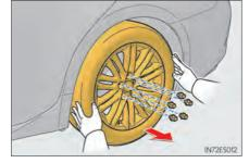
6 Vehicles with a full-size spare tire: Remove the wheel ornament by pushing from the reverse side.
