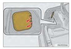
**2** Turn the bulb base counter-clockwise.
