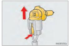
**3** Exchange the light bulb, and install the bulb base.
