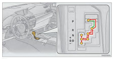
While the "START STOP ENGINE" switch is in IGNITION ON mode, move the shift lever with the brake pedal depressed.
