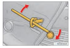
**5** Securely attach a cable or chain to the towing eyelet. Take care not to damage the vehicle body.
