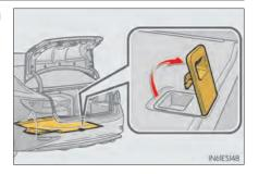
**2** The lever can be hooked on the edge of the trunk.
