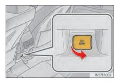
The power outlets can be used when the power switch is in ACCESSORY or ON mode.
