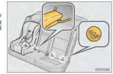
Seat belts equipped with a child restraint locking mechanism (ALR/ ELR belts except driver's seat belt)  $(\rightarrow P.33)$
