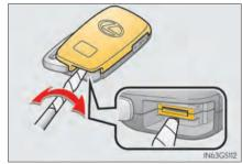
**3** Remove the depleted battery.
