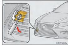
Insert the towing eyelet into the hole and tighten partially by hand.
