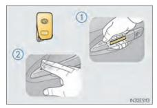
2 Touch the lock sensor (the indentation on the upper part of the door handle) to lock all the doors.
