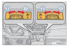
The seat heaters and ventilators can be used when the power switch is in ON mode.
