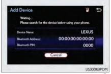
A PIN code are not required for SSP (Secure Simple Pairing) compatible Bluetooth<sup>®</sup> devices. Depending on the device, you may need to select Yes to register, or No to cancel on the device.
