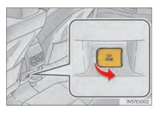
The power outlets can be used when the engine switch is in ACCESSORY or IGNITION ON mode.
