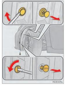
2 While holding the clamp open, pull and remove the tabs and open the fender liner.
