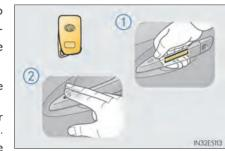
2 Touch the lock sensor (the indentation on the upper part of the door handle) to lock all the doors.
