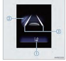
Indicates that steering wheel assistance of the steering control function is operating.
