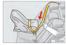
While pushing the child restraint system down into the rear seat, allow the shoulder belt to retract until the child restraint system is securely in place.
