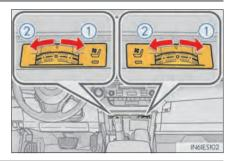
The seat heaters and ventilators can be used when the engine switch is in IGNITION ON mode.
