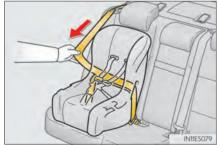
S While pushing the child restraint system into the rear seat, allow the shoulder belt to retract until the child restraint system is securely in place.
