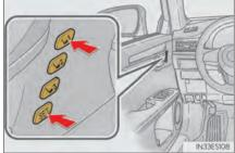
Vehicles with the driving position memory for the front passenger's seat: To record the position of the front passenger's seat, adjust the front passenger's seat to the desired position and perform step 4 using the buttons on the front passenger's side.
