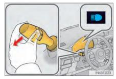
2 Press the Automatic High Beam switch.
