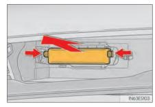
5 Slide and pull out the filter. Replace it with a new one.
