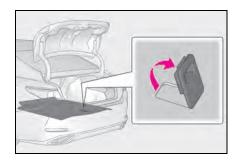
**3** The lever can be hooked on the edge of the trunk.
