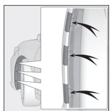
Insert a flathead screwdriver between the front bumper and fender liner and then separate the front bumper from the fender liner.
