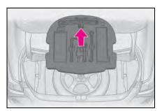
**2** Loosen the center fastener that secures the spare tire.
