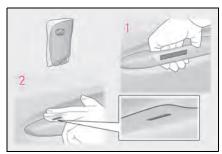
1 Grip the driver's door handle to unlock the door. Holding the driver's door handle for approximately 2 seconds unlocks all the doors. Grip the passenger's door handle to unlock all the doors.\*
