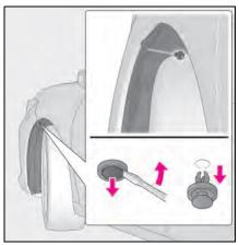
2 To protect the front bumper from being damaged, apply protective tape around the clips as shown in the illustration.
