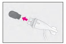
6 Install a new light bulb then install the bulb base to the light unit by inserting it and turning the bulb base clockwise.
