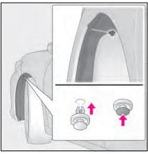
8 Engage the clips to the front bumper to install the fender liner, and then remove the protective tape.
