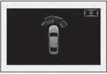
When an object is detected, a graphic will be displayed on the panoramic view monitor (if equipped).
