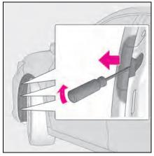
4 Pull back the fender liner and turn the bulb base counterclockwise.
