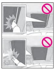
• When using the wireless remote control or mechanical key and operating the panoramic moon roof, operate the panoramic moon roof after checking to make sure that there is no possibility of any passenger having any of their body parts caught in the panoramic moon roof. Also, do not let a child operate panoramic moon roof by the wireless remote control or mechanical key. It is possible for children and other passengers to get caught in the panoramic moon roof.
