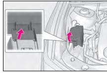
► Engine compartment: type B fuse box
