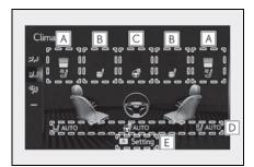
Adjust the seat ventilator fan speed level
