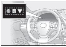
When a tab other than the driving support system information is selected, only a recognized speed limit sign or do not enter sign (when notification is necessary) will be displayed. (→P.71)
