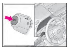
Push the lever away from you with the headlight switch in the AUTO or Dosition.
