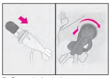
7 Return the fender liner to its original position, and install the clip.
