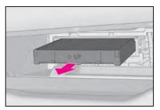
6 Remove the air conditioning filter from the filter case and replace it with a new one.
