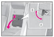
The armrest door can be locked and unlocked using the mechanical key.
