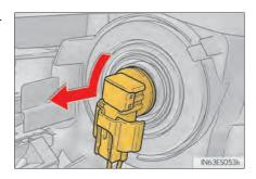
**2** Unplug the connector while pressing the lock release.
