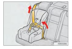
6 If the child restraint has a top tether strap, the top tether strap should be latched onto the top tether strap anchor.  $(\rightarrow P. 68)$
