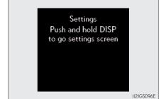
Vehicles without Lexus Display Audio system or a navigation system: Press and hold the "DISP" button after selecting the desired setting item ("Meter", "Vehicle" or "Ambient illumin." [if equipped]) by pressing the "DISP" button.
