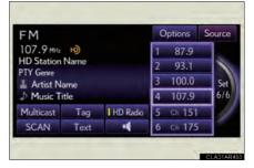
**2** Search for desired stations by turning the "TUNE•SCROLL" knob or pressing and holding " $\wedge$ " or " $\vee$ " on the "PRST•TRACK" button.
