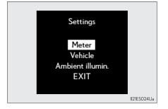
3 Press and hold the "DISP" button after selecting the desired setting item by pressing the "DISP" button.
