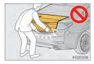
Do not attach any accessories other than genuine Lexus parts to the trunk lid. Such additional weight on the trunk lid may cause the lid to suddenly shut again after it is opened.
