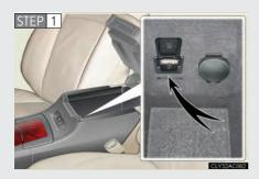
Connect the portable audio device.
