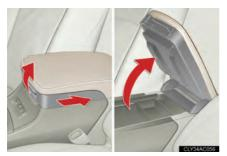
Slide the armrest while pulling up the lever, and lift the armrest.
