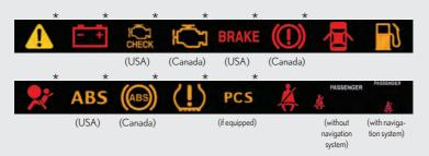
\*: These lights turn on when the "ENGINE START STOP" switch is turned to IGNITION ON mode to indicate that a system check is being performed. They will turn off after the engine is started, or after a few seconds. There may be a malfunction in a system if a light does not come on, or if the lights do not turn off. Have the vehicle inspected by your Lexus dealer.
