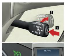
■ Press the "ON-OFF" button to activate the cruise control.
