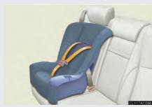
Seat belts equipped with a child restraint locking mechanism (ALR/ELR belts except driver's seat belt) (→P. 59)
