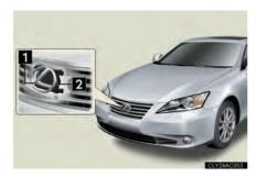
Detects vehicles or other obstacles on or near the road ahead and determines whether a collision is imminent based on the position, speed, and heading of the obstacles.
