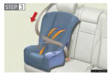
Fully extend the shoulder belt and then allow it to retract slightly into the ALR lock mode.
