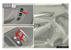
While pressing the desired button (1 or 2), press the lock or unlock side on the driver's door lock switch until the signal beeps.
