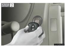
Touch the Lexus emblem side of the electronic key to the "ENGINE START STOP" switch.
