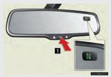
To turn the compass on or off, push and hold "AUTO" for 3 seconds.
