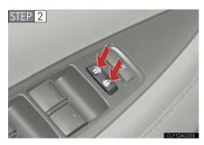
Shift the shift lever to P or N, and press and hold the driver's door lock switch ( or or ) for approximately 5 seconds and then release.
