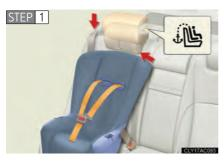
Secure the child restraint using a seat belt or the lower anchors, and lock the head restraint in place at the lowest position.
