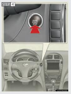
Press the "ENGINE START STOP" switch.
