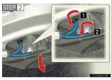
Partly remove the trunk panel cover and turn the bulb bases counterclockwise.
