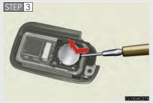
Remove the depleted battery.
