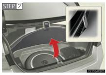
Secure the panel using the hook provided.
