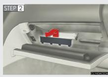
Open the glove box. Remove the glove box cover.
