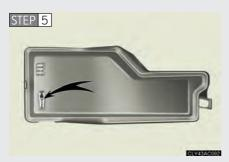
Remove the fuse with the pullout tool.
