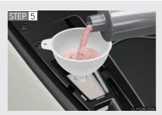
Add engine coolant if necessary.
