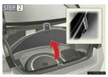
Secure the panel using the hook provided.
