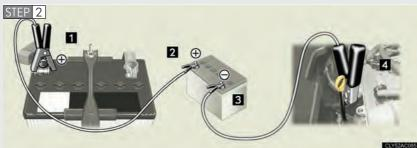
Connecting the jumper cables.
