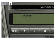
To select the CD to be ejected, press " $\wedge$ " or " $\vee$ " on  $\boxed{\phantom{A}}$  TYPE-DISC  $\wedge$ .
