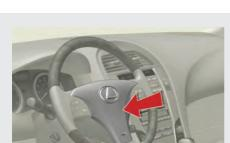
To sound the horn, press on or close to the mark.
