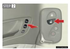
While pressing the desired button (1 or 2), press on the wireless remote control until the signal beeps.
