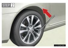
Slightly loosen the wheel nuts (one turn).
