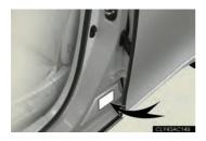
For the GAWR, see the Certification Label. For the maximum load of the tire, see the load limit at maximum cold tire inflation pressure mentioned on the sidewall of the tire.  $(\rightarrow P. 499)$ .
