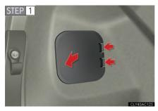
Open the trunk lid and remove the access hole cover.
