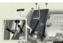
When installing the cover, make sure that the engine coolant reservoir hose positioned as shown in the illustration.
