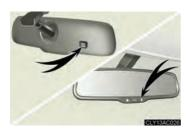
To ensure that the sensors operate properly, do not touch or cover it.
