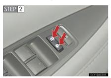
Shift the shift lever to P or N, and press and hold the driver's door lock switch ( or or approximately 5 seconds and then release.
