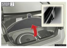
Secure the panel using the hook provided.
