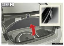
Secure the panel using the hook provided.
