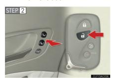
While pressing the desired button (1 or 2), press on the wireless remote control until the signal beeps.
