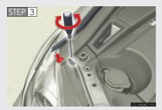
Turn bolt B the same number of turns and in the same direction as step 1 using a Phillips-head screwdriver.
