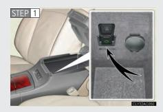
Connect the portable audio device.
