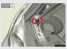
Turn bolt A in either direction using a Phillips-head screwdriver.
