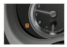
If the vehicle is in danger of slipping, or if the front wheels spin, the slip indicator light flashes to indicate that the VSC/TRAC systems have been engaged.
