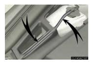
When installing the reservoir cap, make sure that the engine coolant reservoir hose positioned as shown in the illustration.
