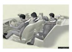
The pretensioner helps the seat belt to quickly restrain the occupant by retracting the seat belt when the vehicle is subjected to certain types of severe frontal collision.
