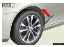
Slightly loosen the wheel nuts (one turn).
