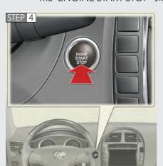
Press the "ENGINE START STOP" switch.
