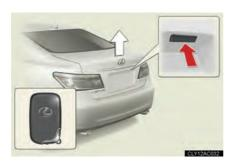
Press and hold the button to unlock the trunk.
