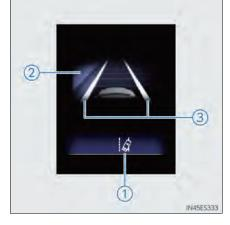
Indicates that steering wheel assistance of the steering assist function or lane centering function is operating.
