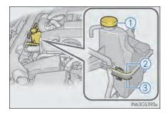
If the level is on or below the "LOW" line, add coolant up to the "FULL" line.  $(\to\!P\!.\,530)$
