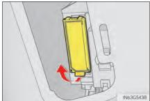
Remove the fuse with the pullout tool.
