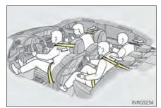
The pretensioner does not activate in the event of a minor frontal impact, a minor side impact, a rear impact or a vehicle rollover.
