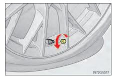
2 Remove the air release cap from the hose.
