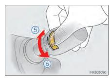
(7) Washer/wiper dual operation Wipers will automatically operate a couple of times after the washer squirts. Vehicles with headlight cleaners: When the headlights are on and the
