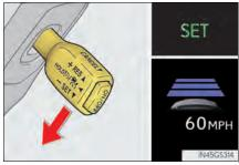
If the lever is operated while the vehicle speed is below approximately 30 mph (50 km/h) and a preceding vehicle is present, the set speed will be adjusted to approximately 30 mph (50 km/h).
