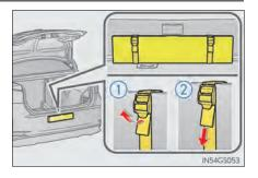
To prevent damage to the warning reflector storage belt when it is not in use, fold the belt (as shown in  $\bigcirc$ ) and secure it with the clip  $\bigcirc$ ).
