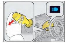
2 Press the Automatic High Beam switch.
