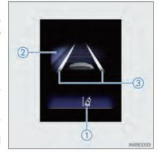
Indicates that steering wheel assistance of the steering control function is operating.
