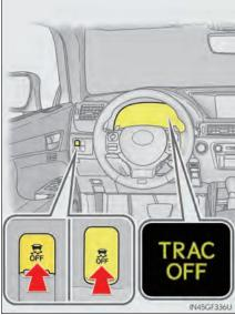
To turn the TRAC system off, quickly press and release  $\cite{1mm}$ .
