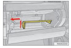
Press the tabs and remove the filter cover.
